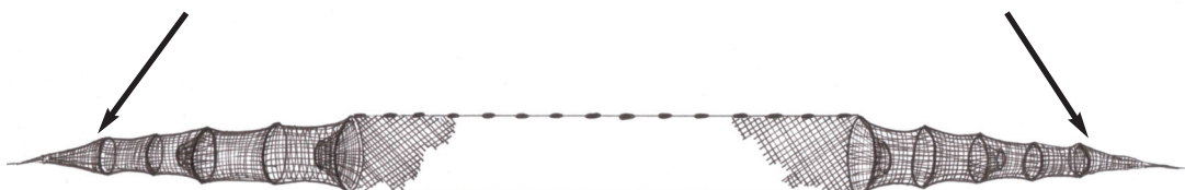
Fig. 2. Schematic drawing of a fyke net. Arrows indicate fish bags, where the catch is gathered.
