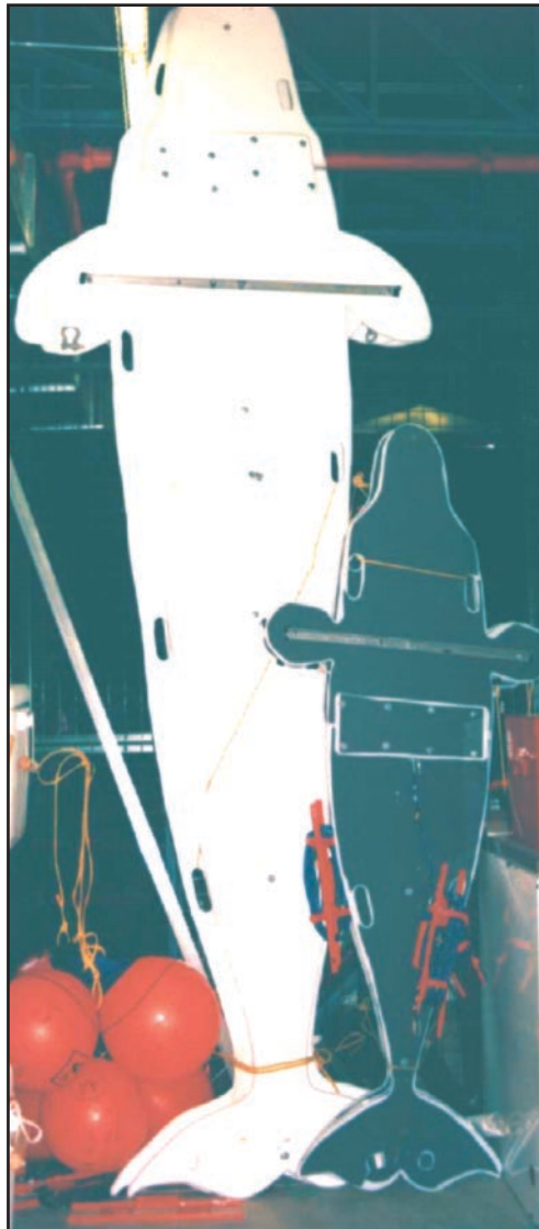
Fig. 2. Beluga models (white adults and grey juveniles) used to estimate the visibility of belugas to aerial photography.
