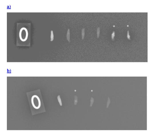
**Fig. 1**. Radiology end point testing of *Shona*'s teeth (a) after three weeks in 10% EDTA, changing the solution every 3-4 days and (b) after an additional two weeks in 10% EDTA. *Shona*'s teeth are highlighted by asterisks and weighed approximately 120 g prior to decalcification.
