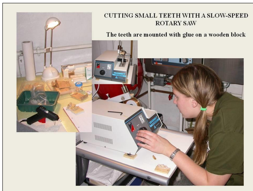
Fig. A3-a1. Set up for cutting and sectioning teeth on a low-speed circular diamond saw.
