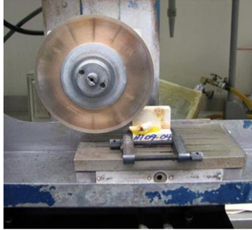
Figure A3-c2. Block carrying mounted tooth through the saw (milling machine).
