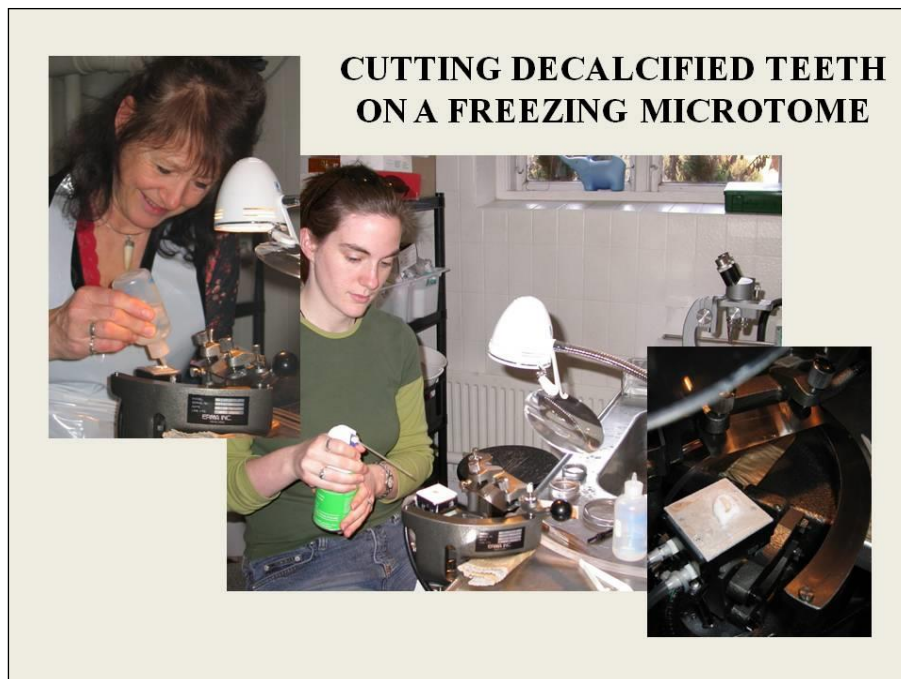
Figure A3-a2. Sectioning a decalcified tooth on a freezing microtome with a fixed freezing platform and movable blade.
