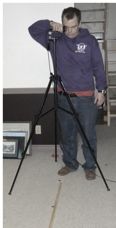
Figure 7. Geometer "sighting in", by making declination measurements from a known Geometer height on target coins at a known distance from the Geometer.
