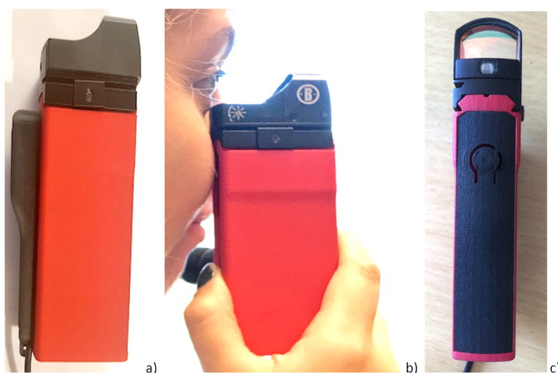
Figure 2. a) 2020 model Pi Geometer with a top-mounted red dot sight (covered) and an armoured USB connector cover; b) 2019 model held in vertical orientation, with sight cover removed; and c) front of the Geometer.
