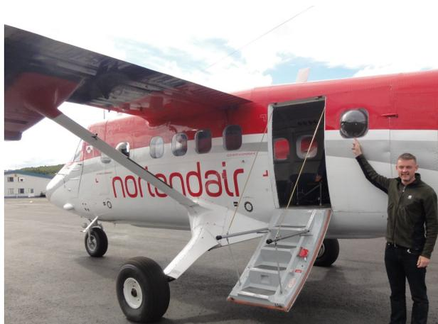
Figure 5. Bubble windows to ensure observers have unobstructed views ahead and under the plane (Photo: R. G. Hansen).
