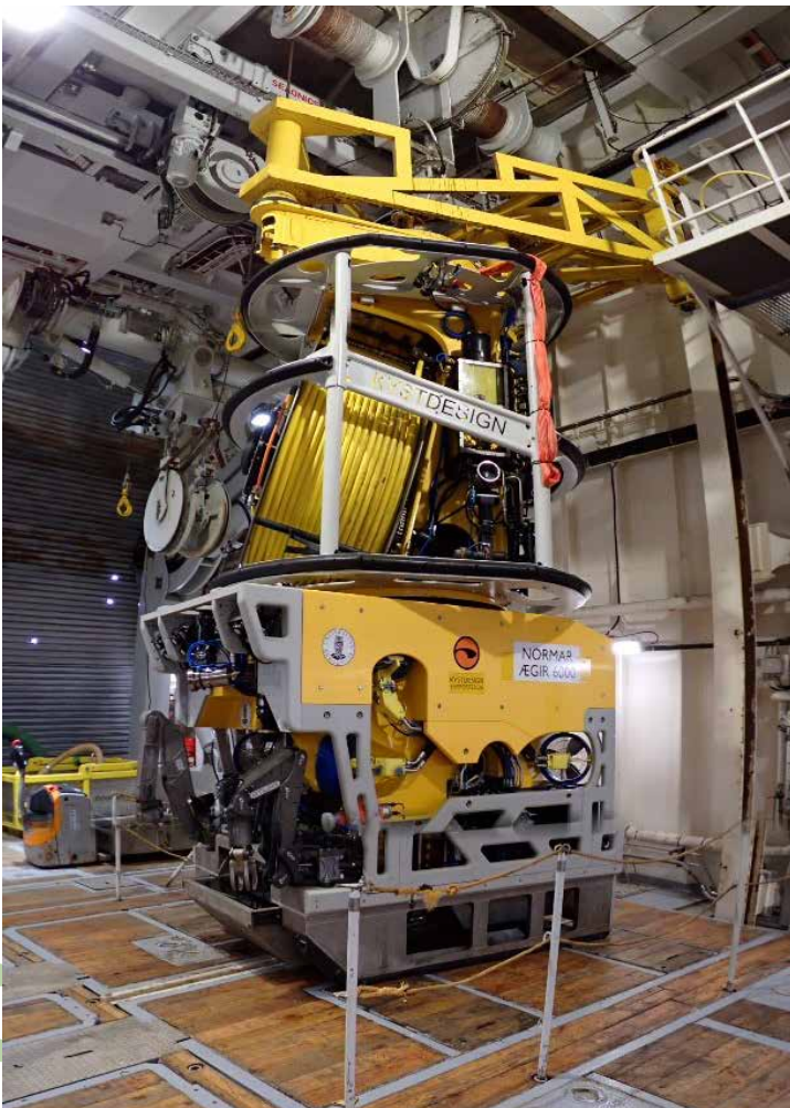
ÆGIR 6000 is a remotely operated vehicle (ROV) designed to be used by scientists to access and study the sea floor. It is suitable for depths of up to 6000 meters. ÆGIR is operated by the Norwegian Marine Robotics Laboratory at the University of Bergen (UiB). Image credit: Solmaz Mohadjer.
