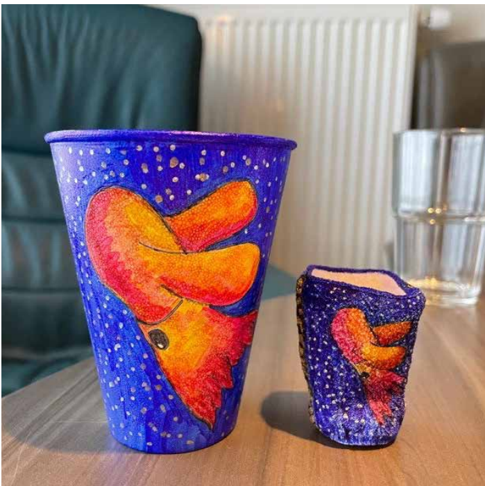
There is a lot of pressure at the bottom of the sea! Comparison of styrofoam cup at normal size and after compression at 4400m depth (Image: AKMA Project)
