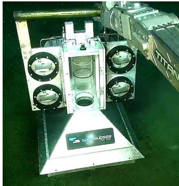
Figure 7. Picture of the gas sampler used during the AKMA3 cruise. The funnel at the bottom has a footprint of 0.5x0.5 m. Gas accumulates in the transparent cylinder atop the funnel. That way, the gas volume can be measured. A valve on the front can be turned and the accumulated gas will evacuate into one of the 4 steel cylinders on the back.
