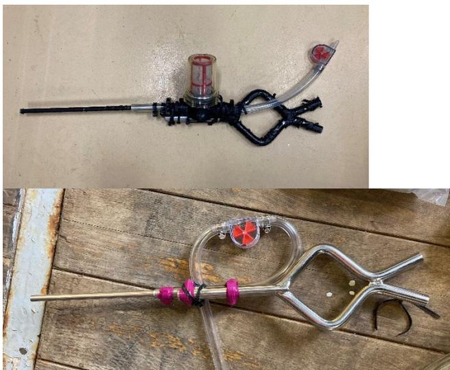
Figure 37. Up: The first version of the sampling wand for SAGE. Bottom: The improved sampling wand for SAGE, including a filter before the spinner.
