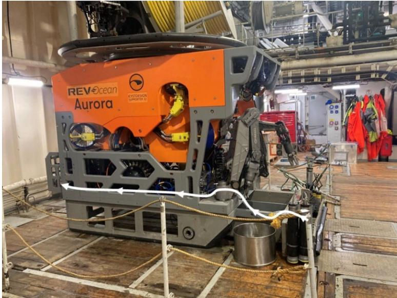
Figure 36. Upper Up: The rear basket of the Aurora ROV, where SAGE was mounted Upper Middle: Detail of SAGE in the basket. The Seabird pump is in the upper left-hand corner and drew water from the tubing and pumped it past SAGE. Bottom: The tubing path from the sampling wand location in the front basket of the ROV to the rear basket.
