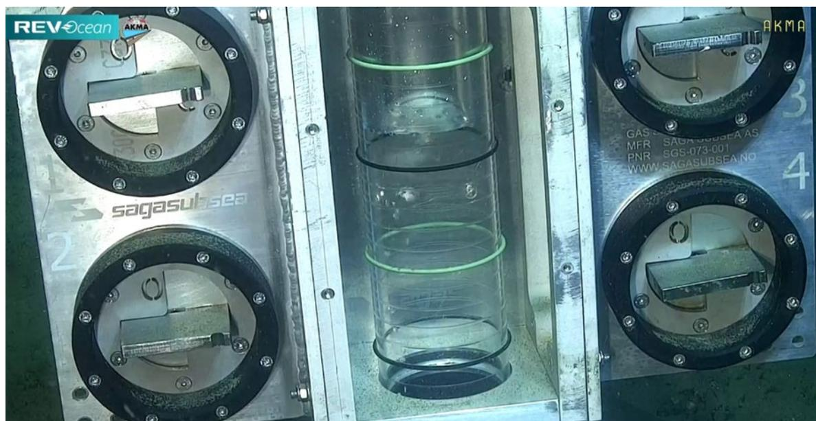
Figure 8. Example of optical-derived gas volume measurements. The green and black markings on the gas cylinder indicate volumes of 0.5, 1.0, 1.5 and 2.0 l respectively. In addition, there are markings every 100 ml in between.
