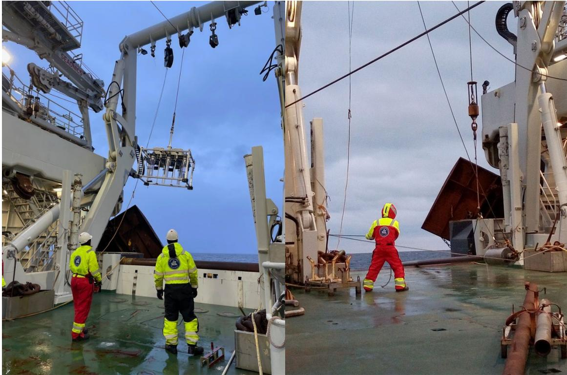
Left: Figure 5. Gravity corer deploying from RV Kronprins Haakon (picture taken during the CAGE22-2 cruise).
