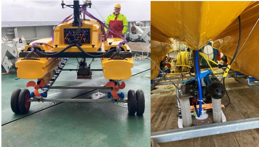
Figure 39. Left: The PAMELi vehicle and SAGE are mounted beneath the vehicle. Right: Close-up of the mounting position of SAGE from the front of the vehicle.
