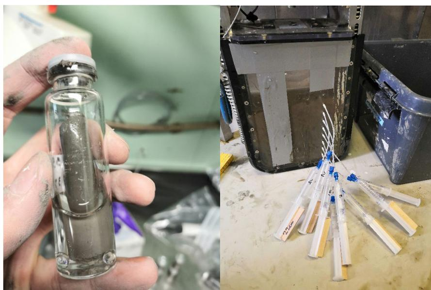
Right: Figure 15. Pore water extraction from a blade core.
