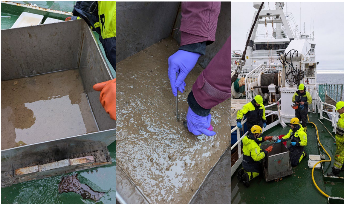
Figure 8. Box core surface, eDNA sampling, and sample processing after siphoning off the water at station 5.
