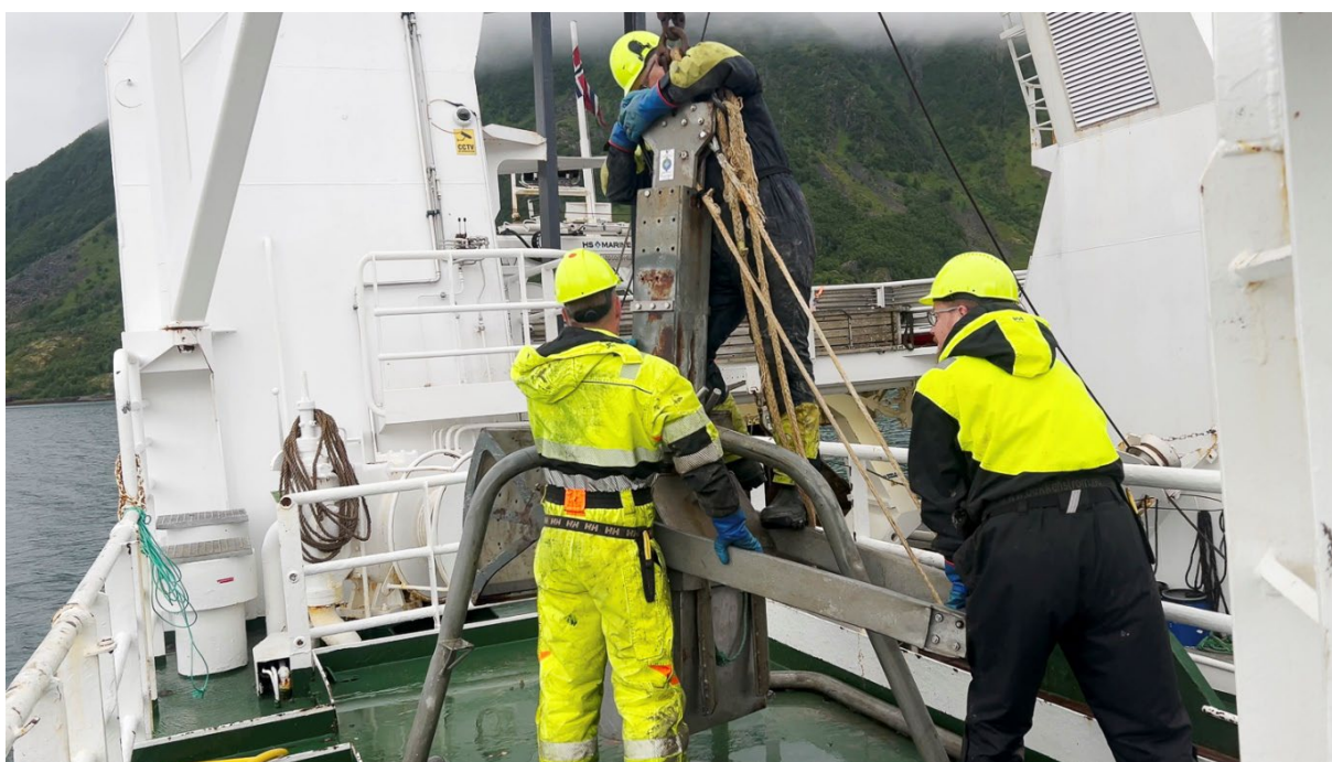
Figure 13. Preparation of the box corer on deck before deployment
