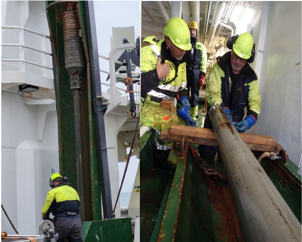
Figure 5. Gravity corer deployed at station 3.
