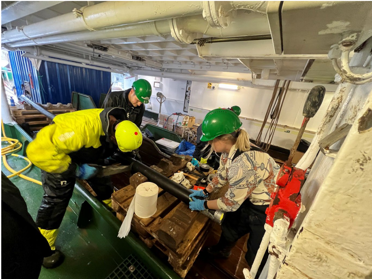
Figure 14. Processing of the gravity core on deck
