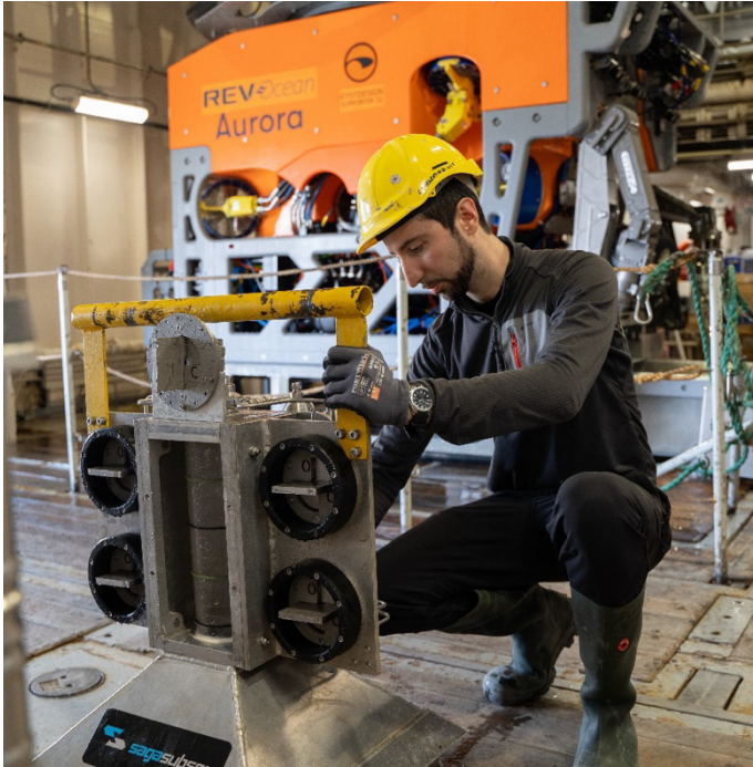
Figure 3. Picture of the gas sampler used during the EXTREME24 cruise. The funnel at the bottom has a footprint of 0.5x0.5 m. Gas accumulates in the transparent cylinder atop the funnel, allowing gas volume measurement. A valve on the front can be turned and the accumulated gas will evacuate into one of the 4 steel cylinders on the back (photo by: Jørn B. Nyvoll).
