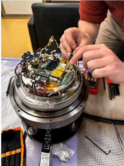
Figure 12. Careful disassembly of SAGE at sea, using ratchet straps to keep the instrument steady.
