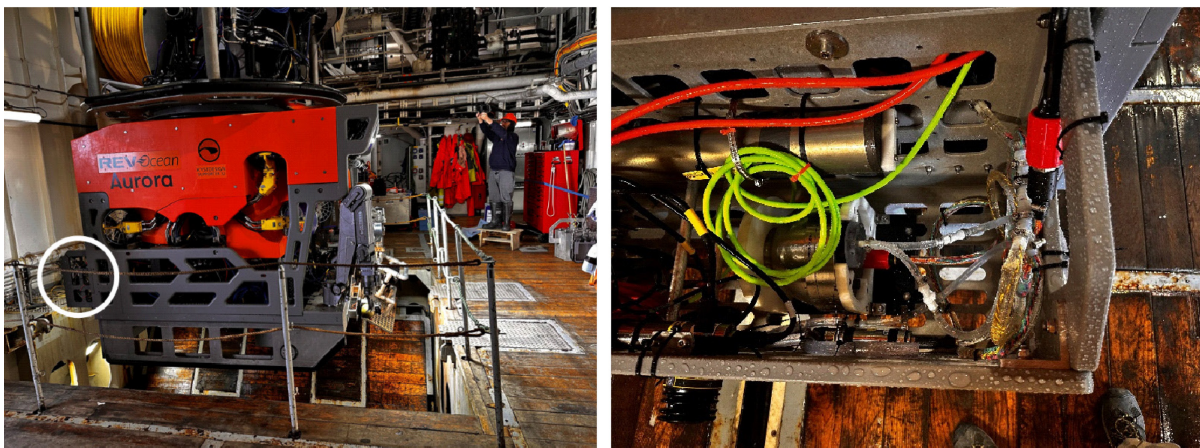
Figure 11. Left: Location of the rear basket on the ROV Aurora. Right: SAGE mounted in the basket.
