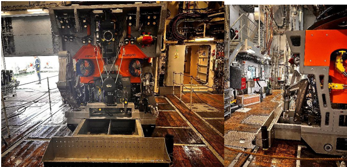
Figure 14. Left: High MISO camera mounting position, showing the full vehicle. Right: MISO camera position, showing angling of the camera downwards to better capture the seafloor. The angle of tilt was adjusted throughout the deployment process to optimize the view of the seafloor.
