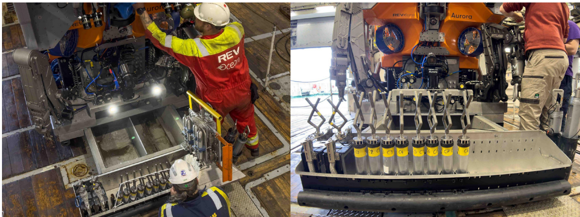
Figure 5. Sampling tools arrangement on ROV Aurora during EXTREME24 (photo by: Jørn B. Nyvoll).
