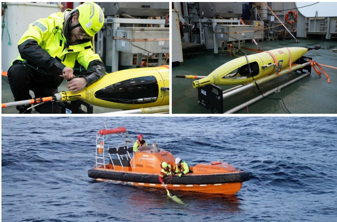
Figure 41. Field technician Sondre Pedersen from Akvaplan-niva assembling sensors onto the Kongsberg glider (upper left and right). Pedersen and crew members deploying the glider in Erik Eriksensstretet (bottom). Photos by Daniel Albert, SINTEF/GoNorth.
