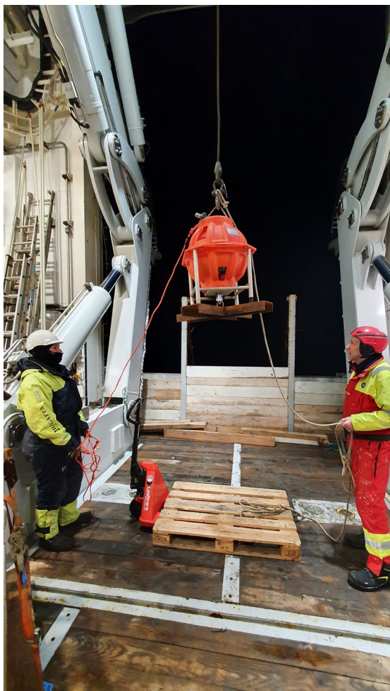
Figure 9. Deployment of Sercel MicroOBS Plus through the A-frame in the main hangar used at the OBS stations GEUS 1–18 (left), and the UiB Ægir6000 remotely operated vehicle (ROV) used for OBS deployment at the station UiB1–5 and GEUS 19 (right). Photos by Thomas Funck, GEUS.
