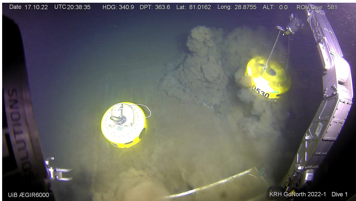
Figure 10. Deployment of University of Bergen's Ocean Bottom Seismometers (OBS) UiB1E and UiB1W using remotely operated vehicle (water depth 364 m). Photo by Ægir 6000/NORMAR.
