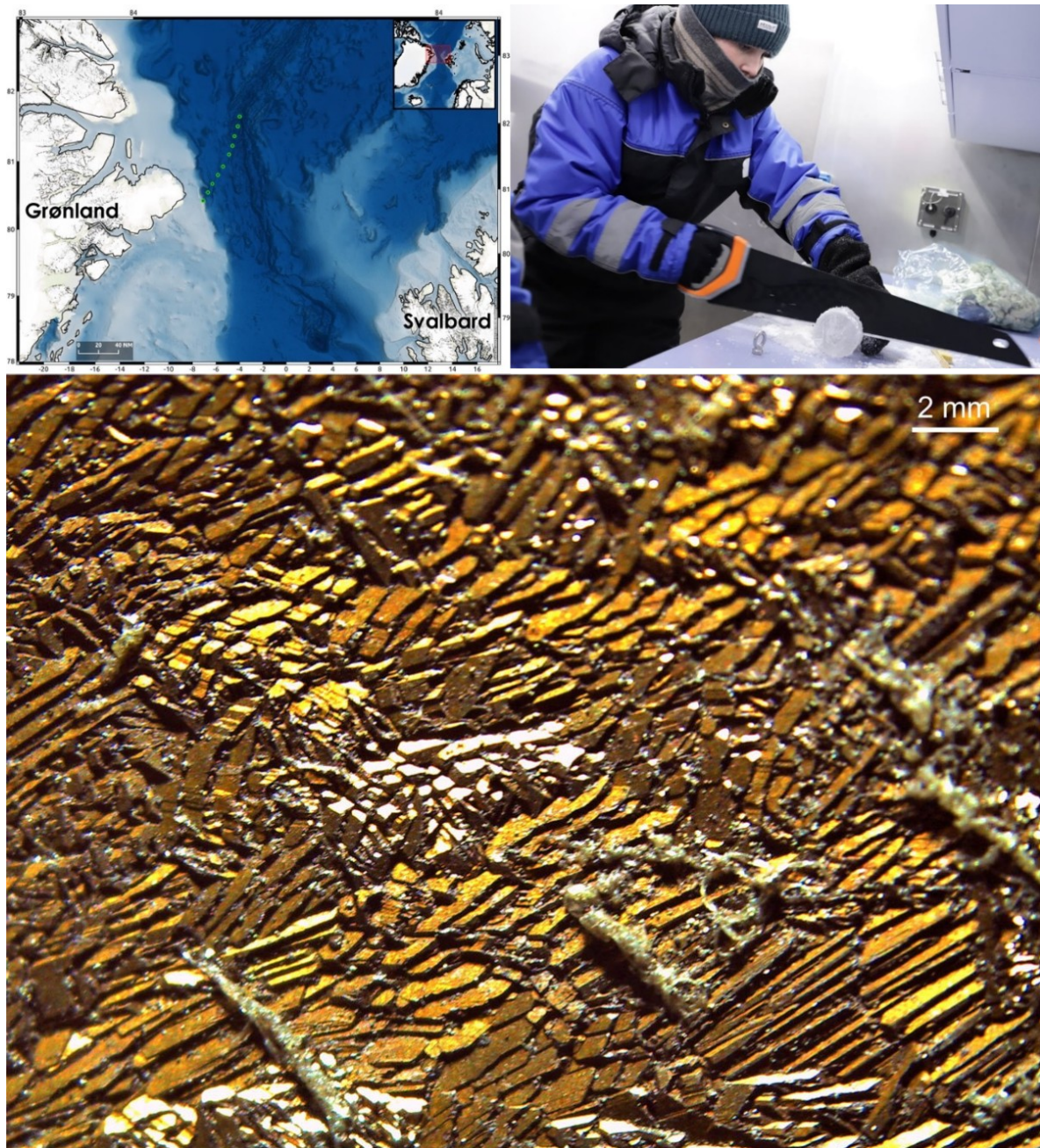
Figure 18. The green dots in the map (top left) show the locations of water samples and CTD measurements. Renée Mie Fredensborg Hansen (NTNU) dividing an ice core sample in the -15^{\circ}\text{C} laboratory (top right). A close up image of the inside of a hydrothermal chimney (bottom). The walls of this chimney are primarily composed of the minerals pyrrhotite and chalcopyrite — indicating fluid temperatures above 300^{\circ}\text{C} . Photos by Daniel Albert, SINTEF/GoNorth (top right) and Sabina Strmic Palinkas, UiT (bottom).
