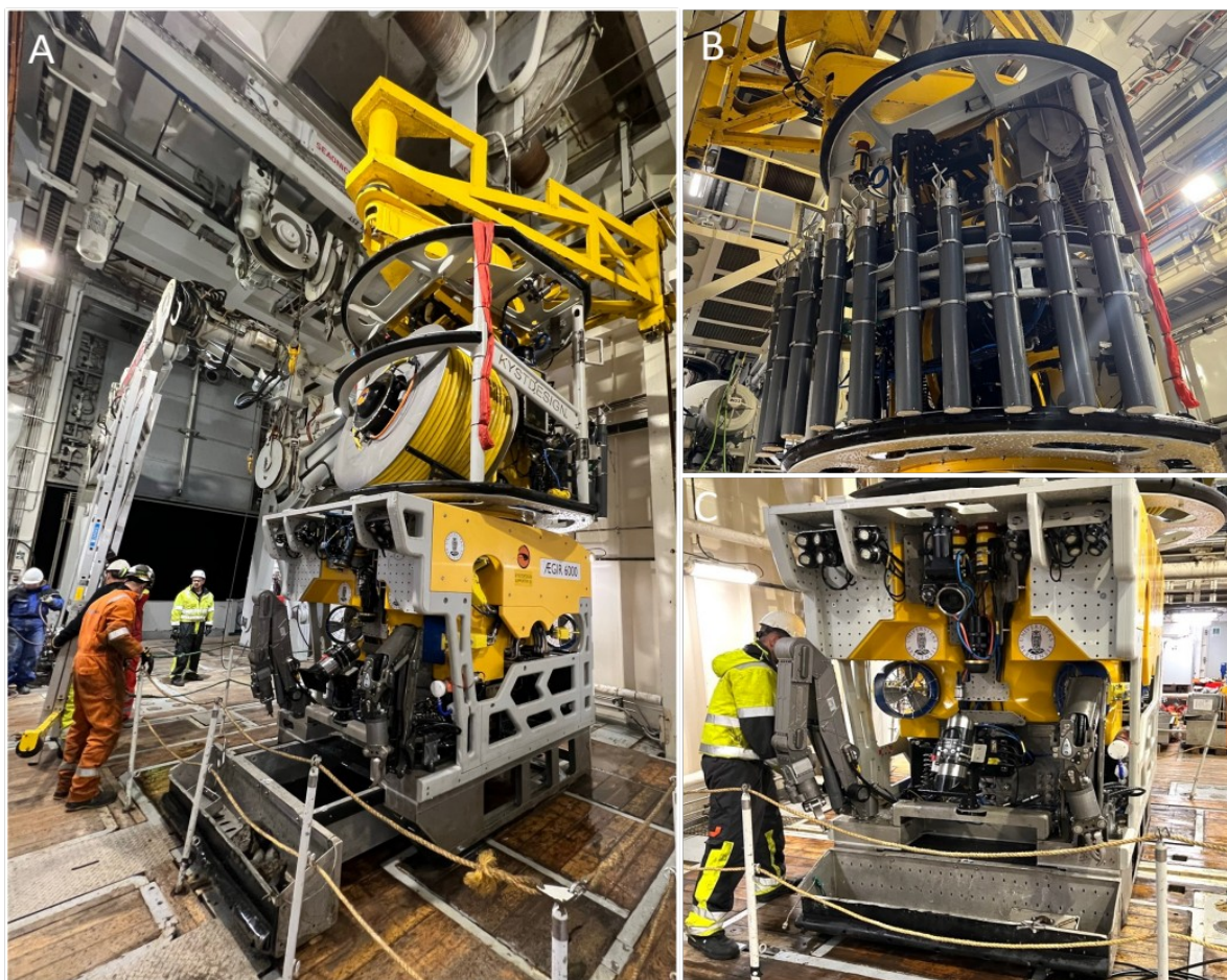
Figure 28. A) The Ægir 6000 in the main hangar of RV Kronprins Haakon standing on the closed hatches of the moon pool. Mounted on top of the ROV is the tether management system (TMS), with a part of the cursor system visible above it. This system guides the ROV and TMS through the moon pool. B) The TMS equipped with a rack of sediment corers attached, showcasing the tooling capabilities of the system. C) The front of the ROV, featuring manipulators, cameras, and lighting, essential for deep-sea exploration and sample collection.
