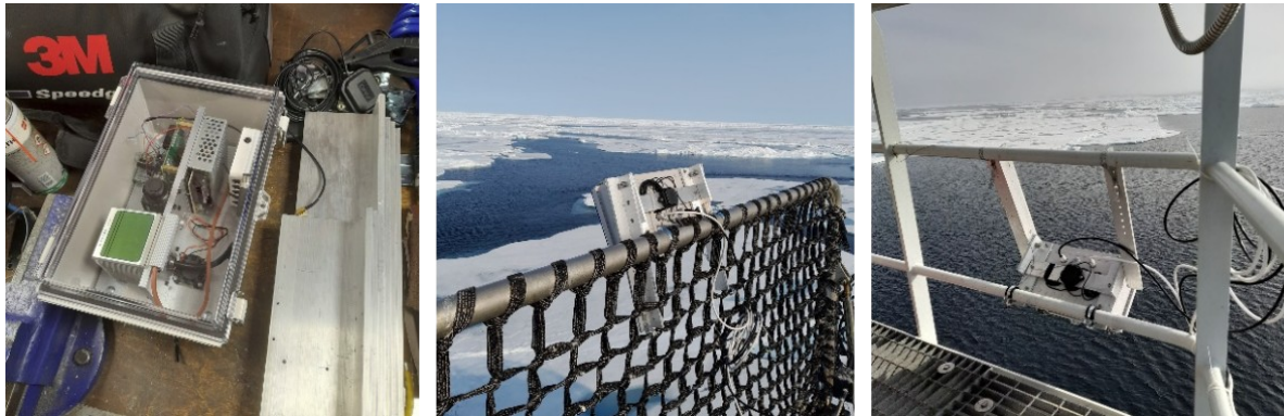
Figure 47. (Left) Inside view of the sensor platform. On the left side, from bottom to the top is the lidar (Livox Mid-70), camera (Blackfly GigE) and navigation module (Aceinna OpenRTK). On the right side is all supporting equipment including a small fan, heating element, network switch and a 12V power transformer. (Center) sensor mount points on the front of the bow, and (Right) sensor mount pointing outside the bridge (on starboard side).
