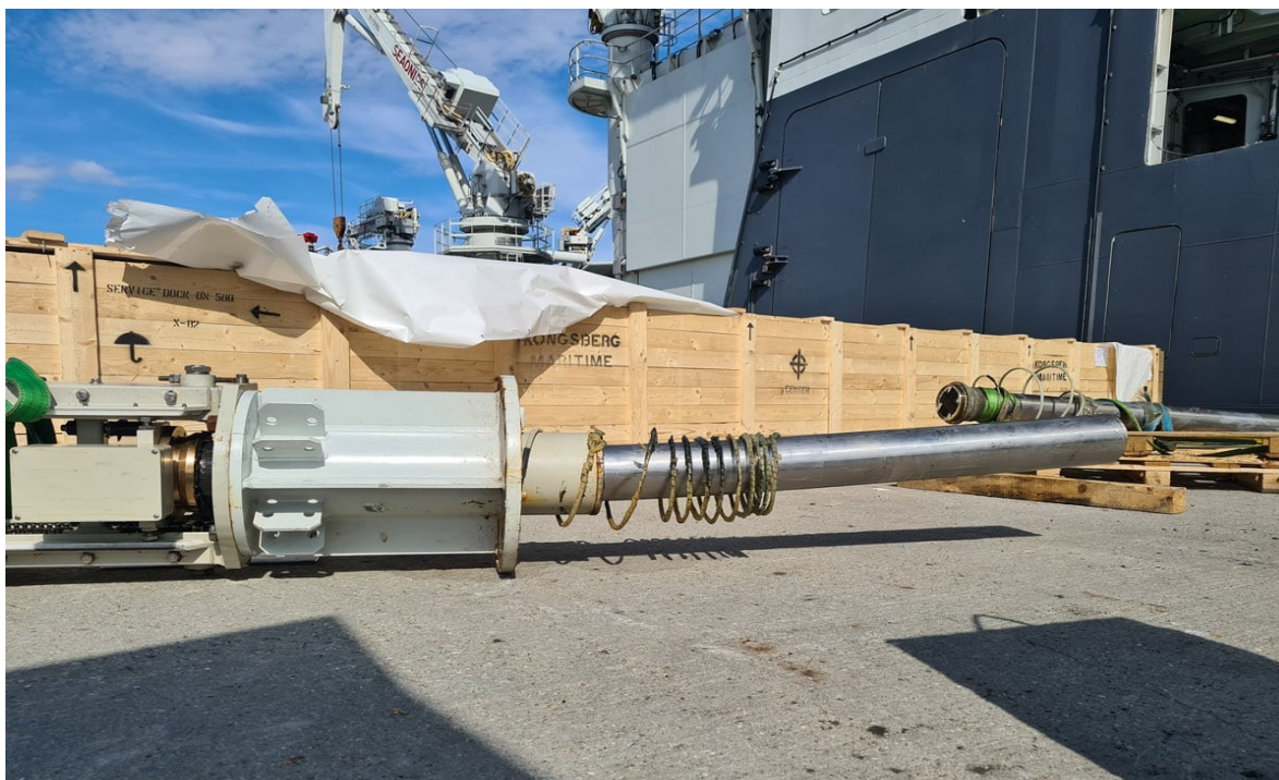
Figure 9. The bent HiPAP steel tube after being removed from the ship. The part that was cut off by the divers is seen in the background to the right. Photo by Daniel Albert, SINTEF/GoNorth.
