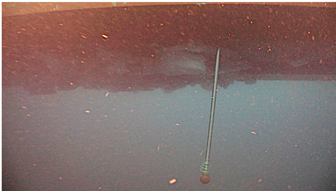
Figure 6. The tube that was bent by the ice, even with its weight of 1.5 tons and diameter of 15–20 cm. In the top of the photo the hull of the ship is visible, the steel tube is 4 m long with the HiPAP-instrument (red sphere) at the end. Normally the tube should be vertical. Photo by Ægir 6000/NORMAR.
