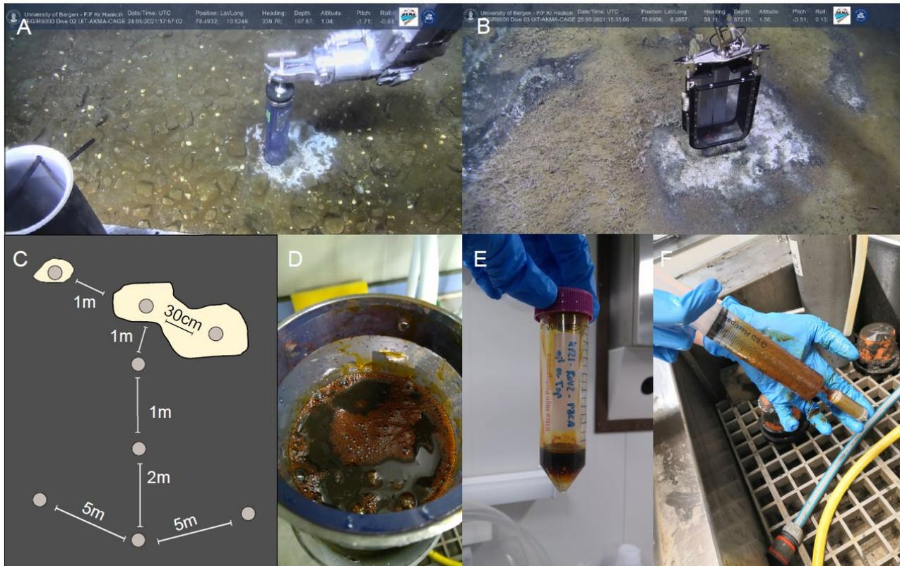
Figure 11 (A, B) Microbial mat covered sediments are sampled by the ÆGIR6000 TITAN4 with push cores and blade cores. (C) sampling strategy at Superstation 2; white marks represent the microbial mat; grey circles represent the push cores sampling location; approximative distances between sampling locations are indicated. (D, E, F (by Claudio Argentino)) Sampling of the push cores taken at Superstation 1.
