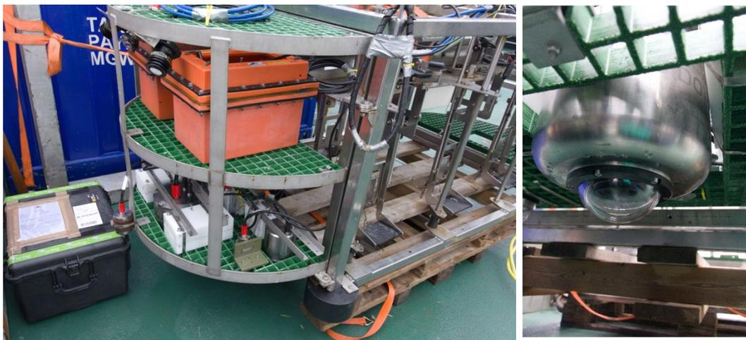
Figure 6: Front of the Deep-tow camera system (on the left), showing front facing camera, bottom facing camera, strobe lights and a battery pack. A detailed view of the pressure housing holding Nikon D810 bottom-facing camera is on the right.
