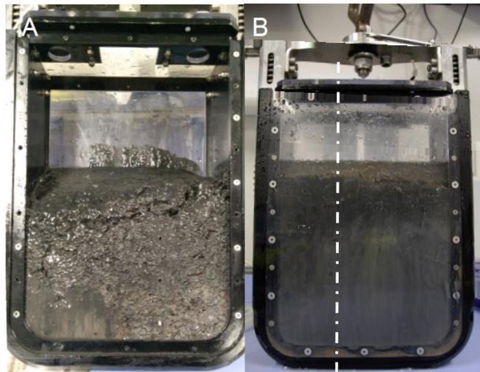
Figure 38: (A) Blade cores taken in a microbial mat covered area and (B) on the edge between tube worms hosting sediments and inactive sediments; the white dotted line indicates the separation between tube worms covered area and adjacent reference sediments.
