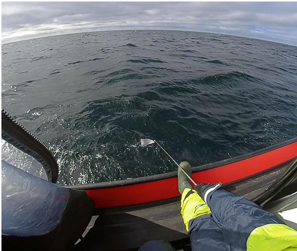
*Figure 10 Surface sampling for spilled oil with the special membrane attached on the telescope. (photo: Maximilian Weber, May 2021)*
