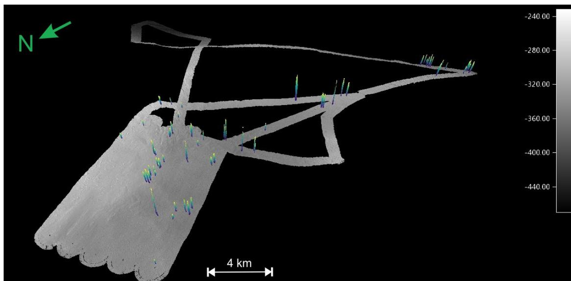
Figure 43: 3D map of the multibeam survey at SS5, highlighting the flares that were extracted from the raw multibeam data. The depth of the bathymetry map is indicated based on a grey scale (m). The mapped gas flares are displayed as vertical features in a colour scale from purple to yellow.
