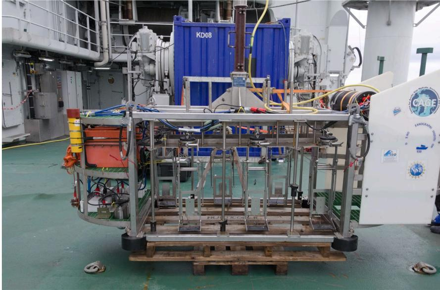
Figure 5: CAGE Deep-tow camera system in preparation for test deployment during CAGE21-1 cruise.
