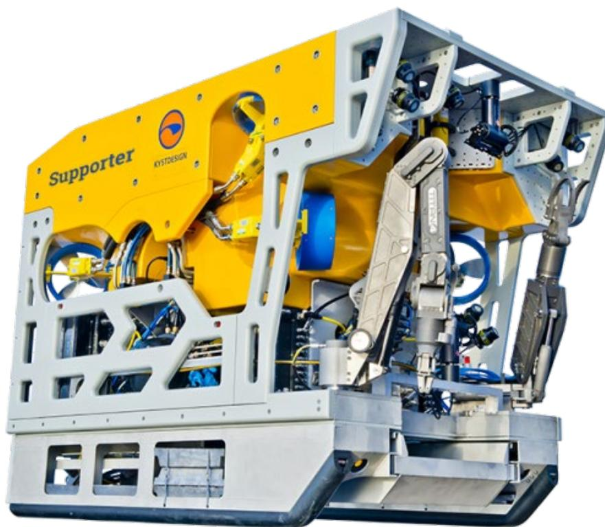
*Figure 7 The ROV Ægir6000 is a Kystdesign Supporter ROV rated to 6000 m water depth.*
