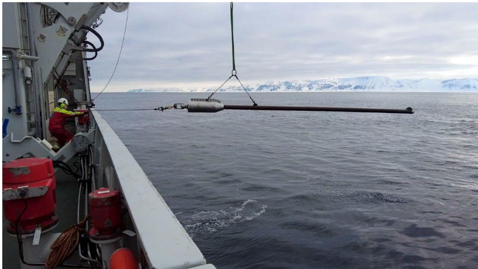
*Figure 2: Gravity corer deploying*
