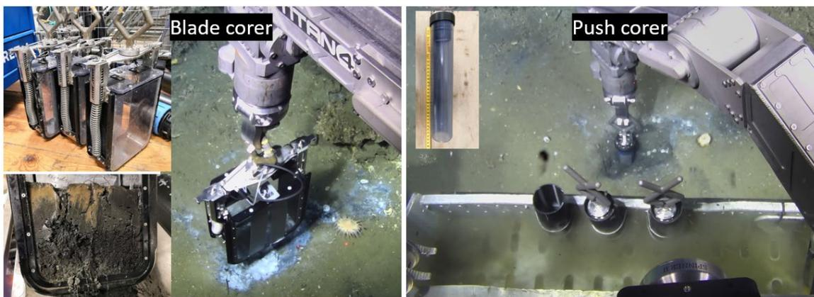
*Figure 8 Blade corer (on the left) and push cores (on the right). The sampling tools are moved by the manipulators of the Ægir ROV. The blade corer has a closing system which prevents sample loss upon recovery and makes it a good sampling tool for fine to coarse sediment. The push coring works fine in clayey “sticky” sediments, but it is inappropriate for sampling of coarser sediments.*
