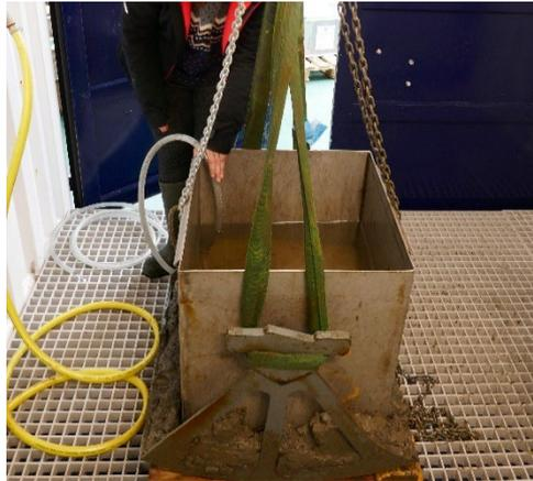
*Figure 3: Box corer full of sediment ready to be processed*
