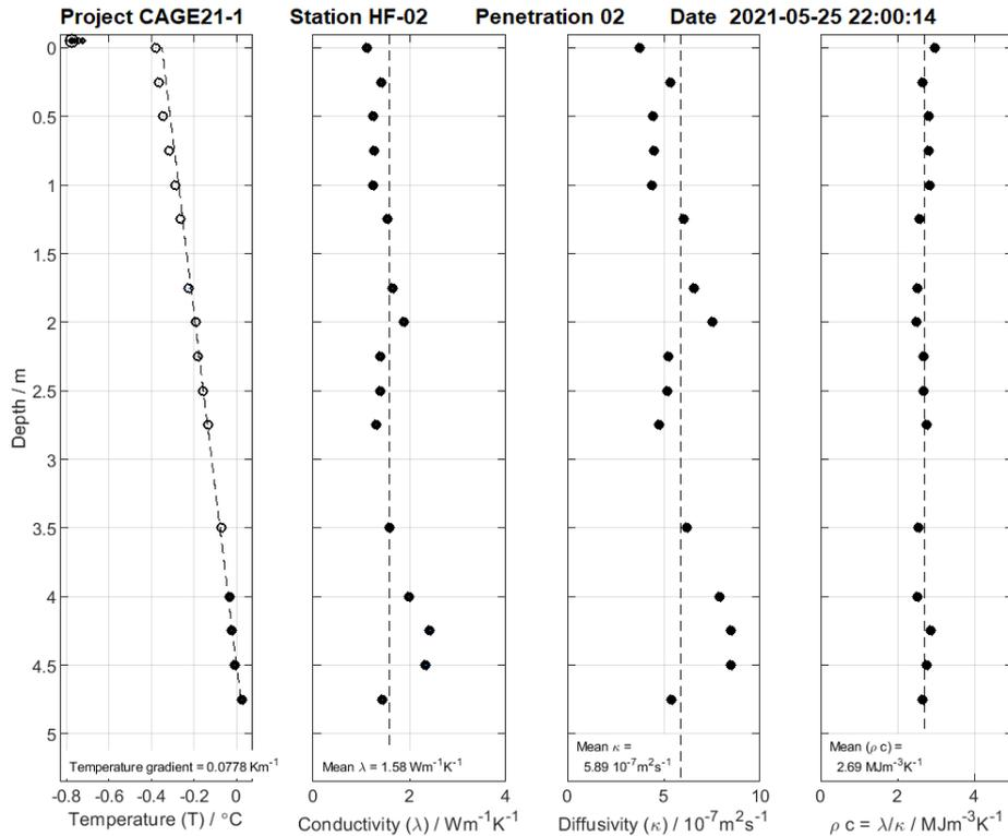
Figure 28: Plot of temperatures and thermal properties measured at station HF-02-02. Higher thermal conductivities are observed at 4.0 – 4.5 m below the seafloor.
