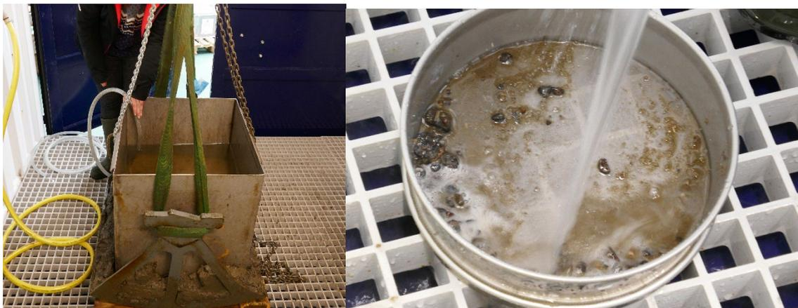
*Figure 13 Box corer full of sediment and sediment being sieved for facilitate observations under the binocular microscope. Credits: Max Weber.*
