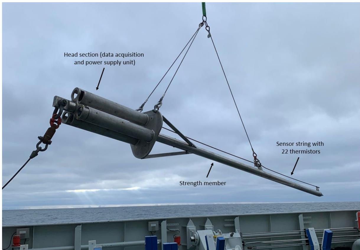
*Figure 4 The Fielax heat flow probe being deployed from RV Kronprins Haakon during the CAGE21-1 cruise*
