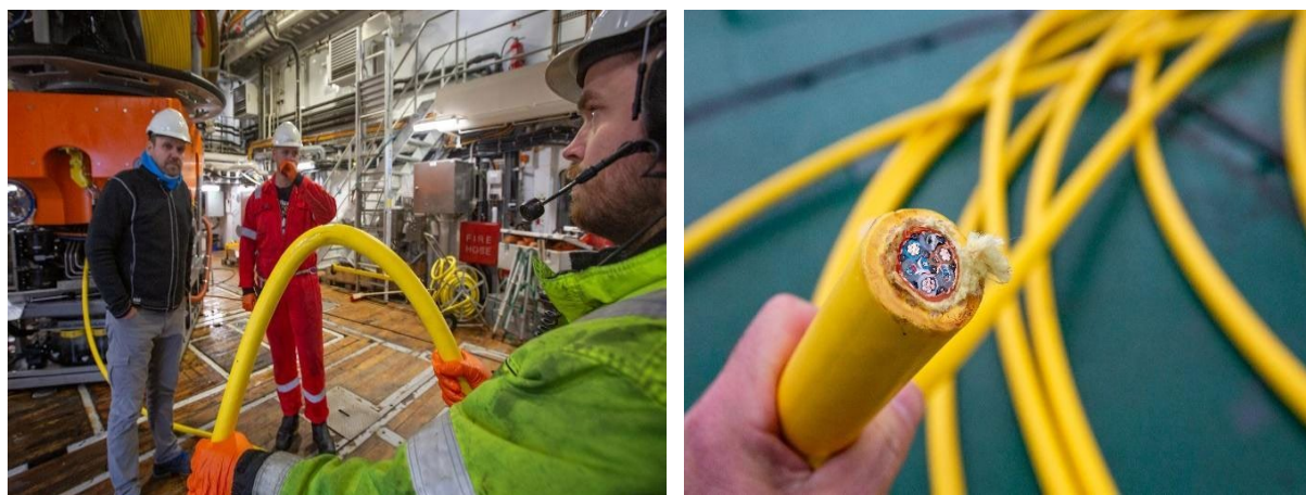
Figure 17. Repair of the ROV's umbilical tether.
