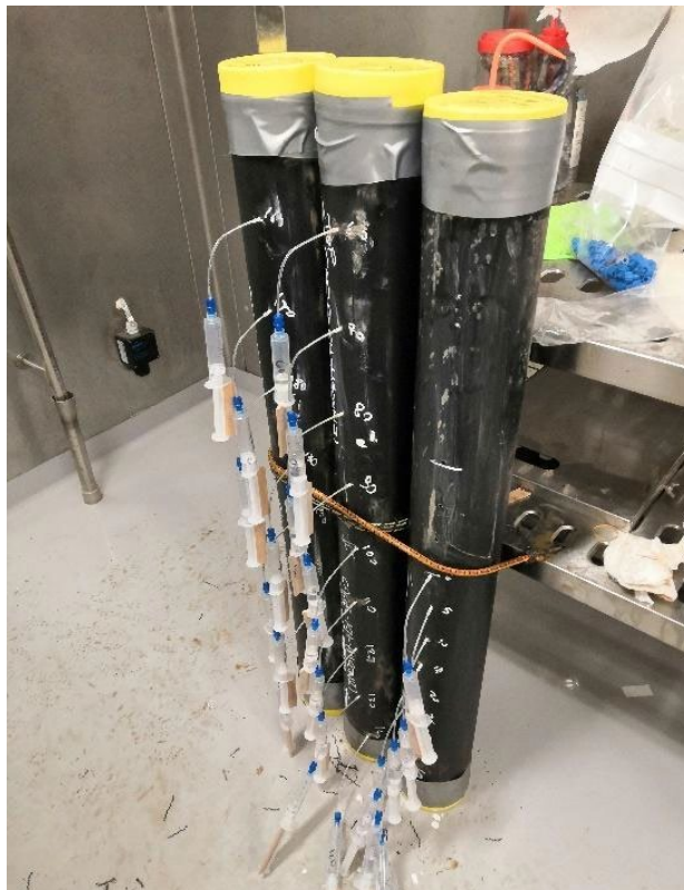
Figure 33. Pore-water sampling of gravity core CAGE-KH-HACON21-02-GC-193
