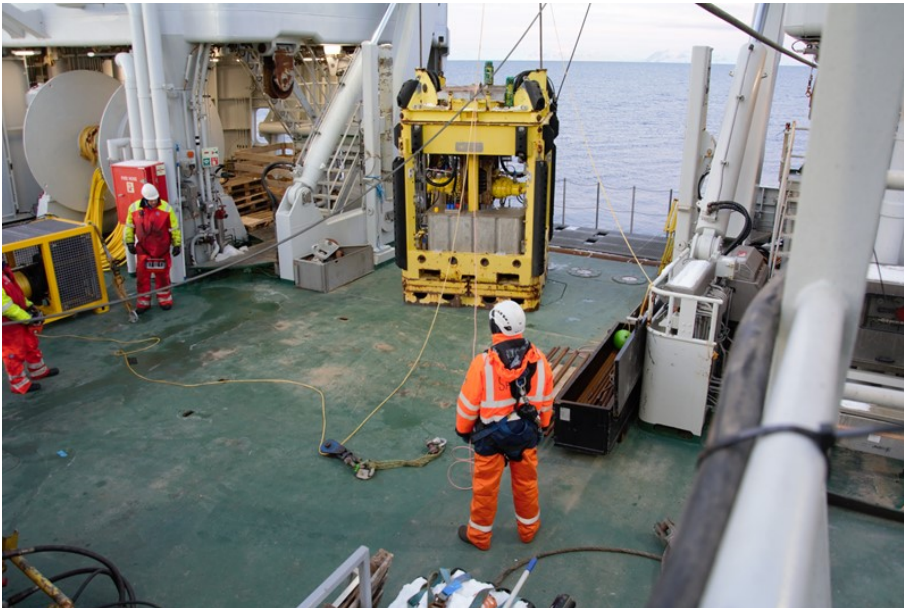
Figure 3: Manta-200 on deck on R/V Kronprins Haakon in preparation for deployment offshore.
