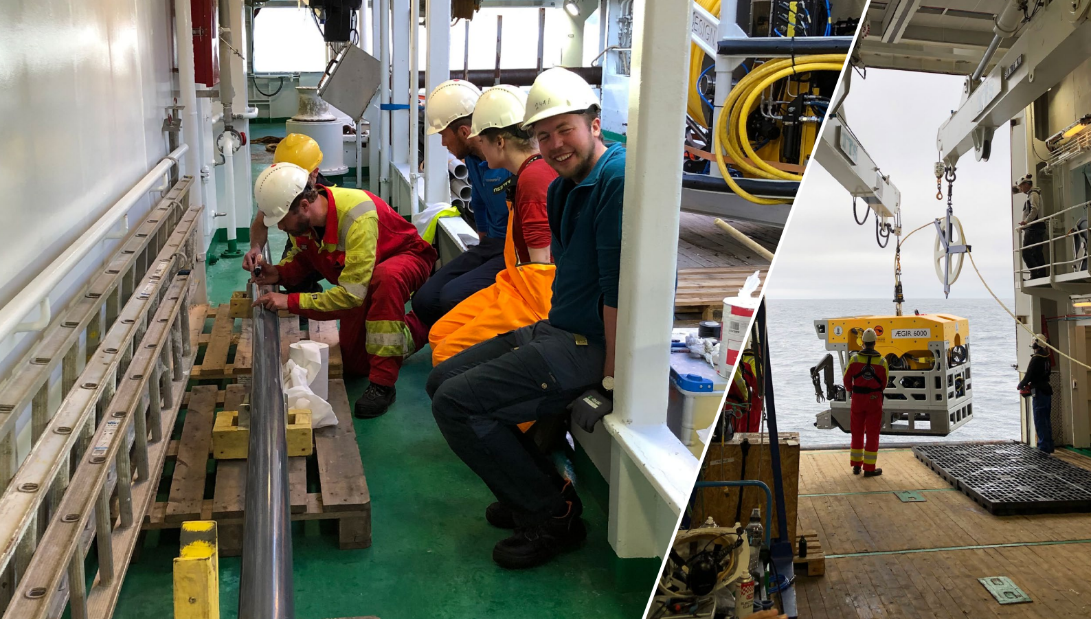
Sediment coring of seep sites on the Mid-Norwegian shelf onboard RV "G.O. Sars". Launching of ROV ÆGIR 6000 from RV "G.O. Sars". Photos: Jochen Knies
