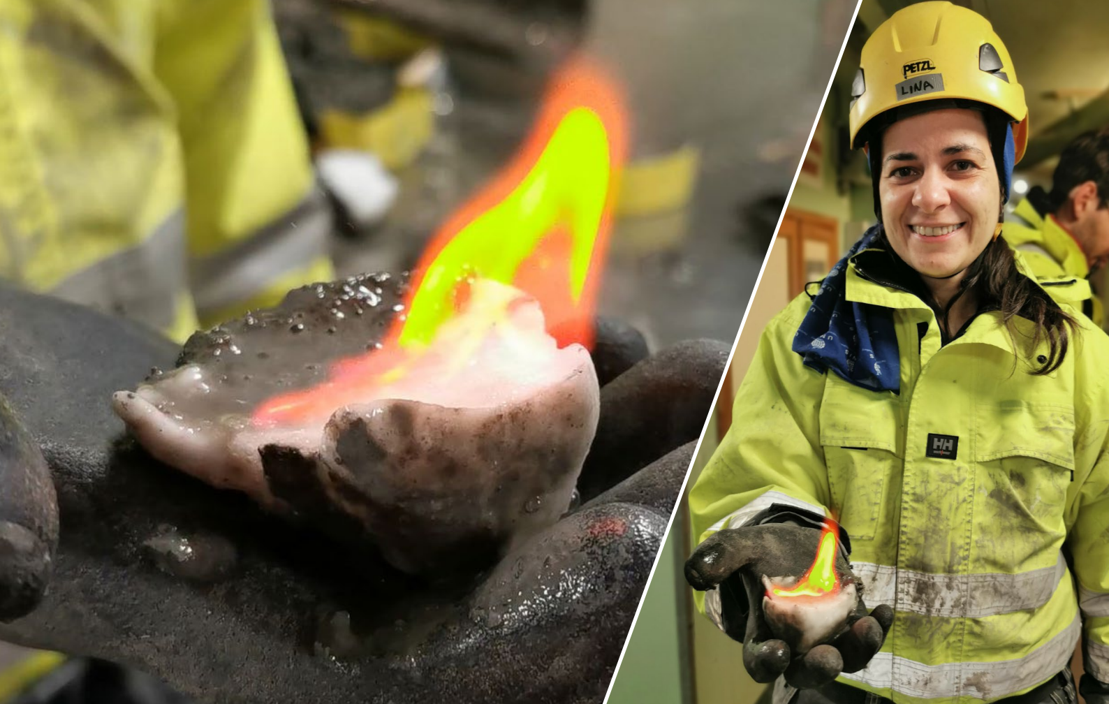
Burning ice: gas hydrate retrieved in a core from the central Barents Sea. PhD student Nikolitsa Alexandropoulou holding burning gas hydrate sampled in the central Barents Sea. Photos: Henry Patton
