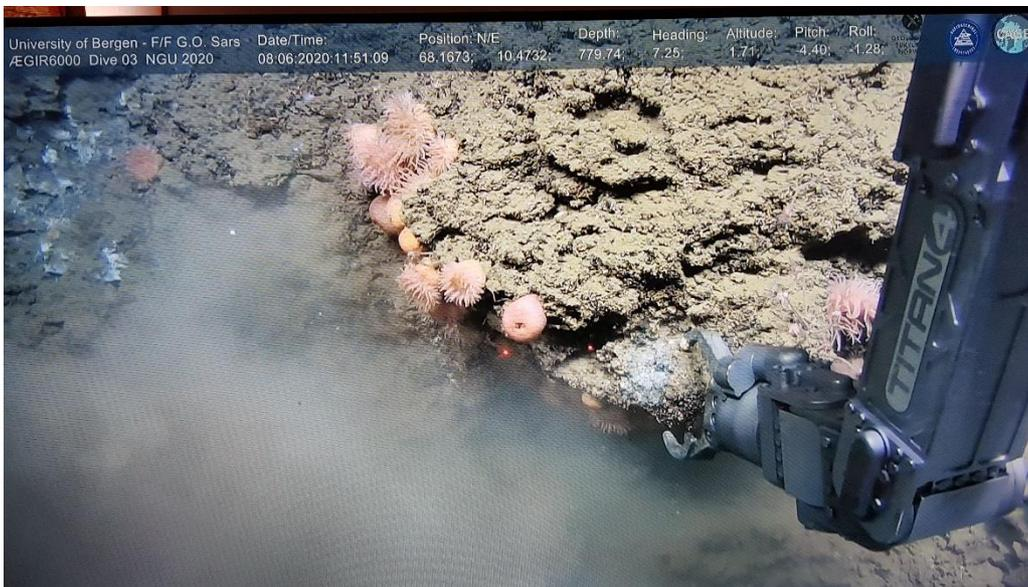
**Figure 11.** ROV bedrock sampling in Canyon North ores (yellow) and rock samples (purple).
