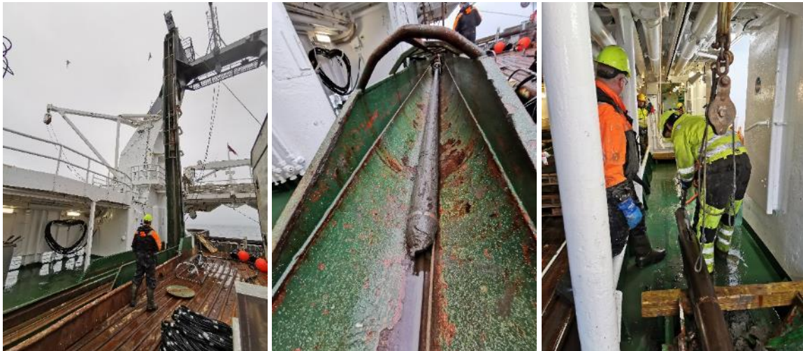
Figure 6: A) Gravity core being raised onto deck; B) Successful recovery of sediments by the corer; C) Removing the core liner prior to preparation for cold storage. (Photos: H. Patton).
