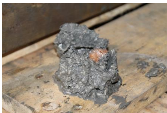
Figure 25: Hydrate flakes recovered from the core-catcher of GC352 and set alight. (Photo: N. Alexandropoulou).
