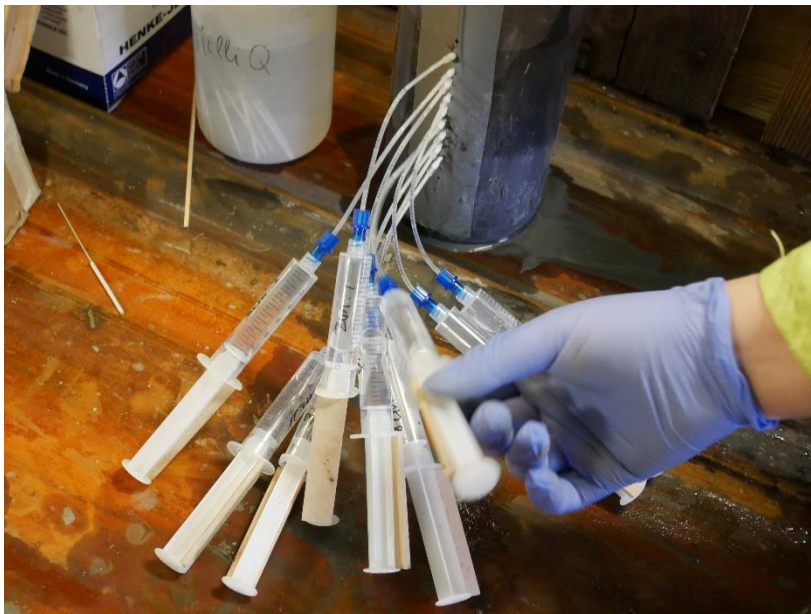
Figure 4 Pore water extraction from a push core collected from a box core. Rhizons are inserted every cm and water is collected into 10 ml syringes. Photo credits: Selina Bernd.
