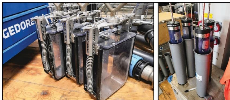
Figure 8. Blade corers (left picture) (frame 25 x 10 x 32 cm) and push corers (right picture) (inner diameter 8 cm, length of 60 cm) used during visually-guided sediment sampling with the ROV.
