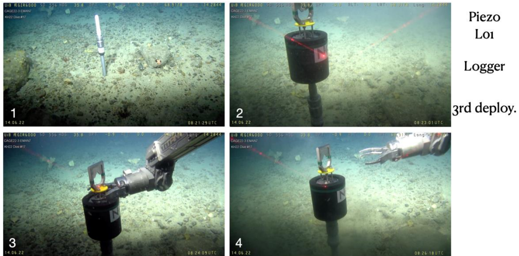
Figure 16. Deployment of the piezometer L01 Logger using the ROV (3 rd deployment). Dive #17, 14/06/22, 0826am. 1: standpipe; 2: logger positioned on the standpipe; 3: pushing on the logger; 4: logger is deployed, and piezometer is complete.
