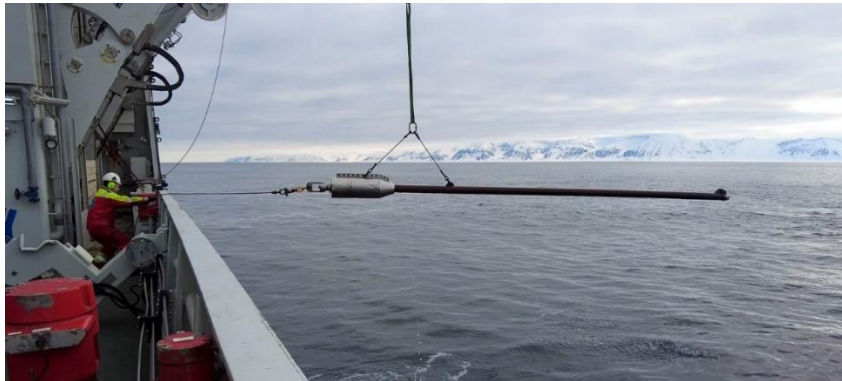
Figure 9. Gravity corer deployment from RV Kronprins Haakon.
