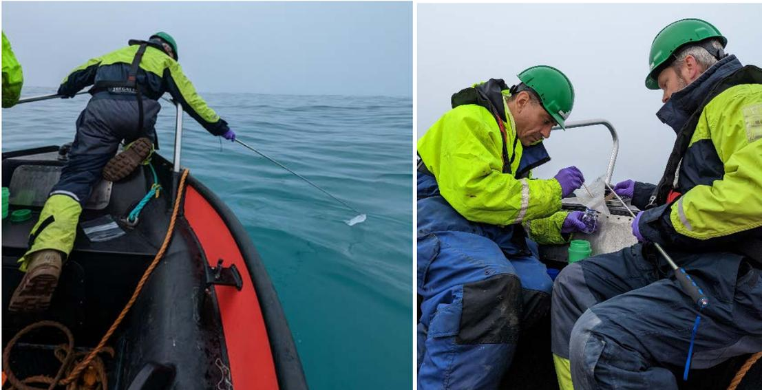
Figure 9: Sampling oil slicks from the working boat using a ETFE membrane at station 1248 (Photos: H. Patton).
