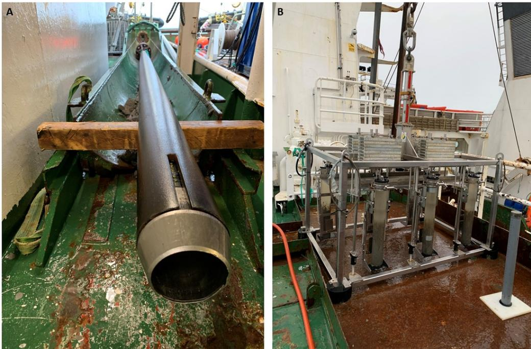
Figure 7: Sediment sampling equipment. A – gravity corer; B – multi corer
