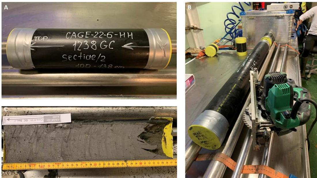
Figure 8: Sediment core processing. A – core liner cut in sections; sections are labelled and sealed. B – core liner ready for splitting with a rotary saw. C – split open core section ready for subsampling and description.
