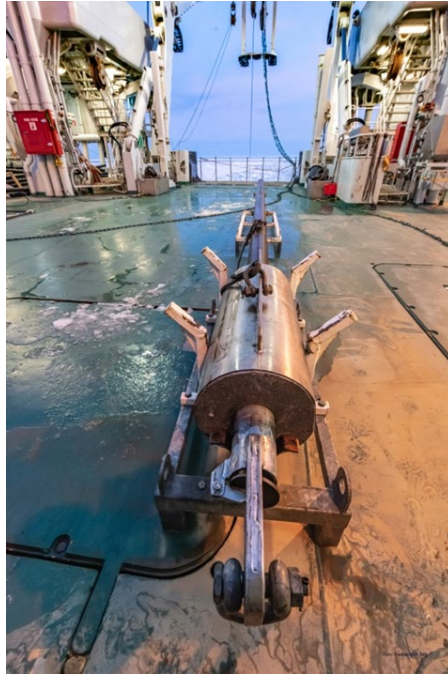
Figure 10.3. Gravity corer used during HACON19 expedition.
