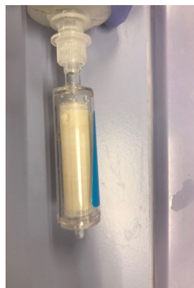
Figure 12.3. Sterivex filter from a bottom section.
