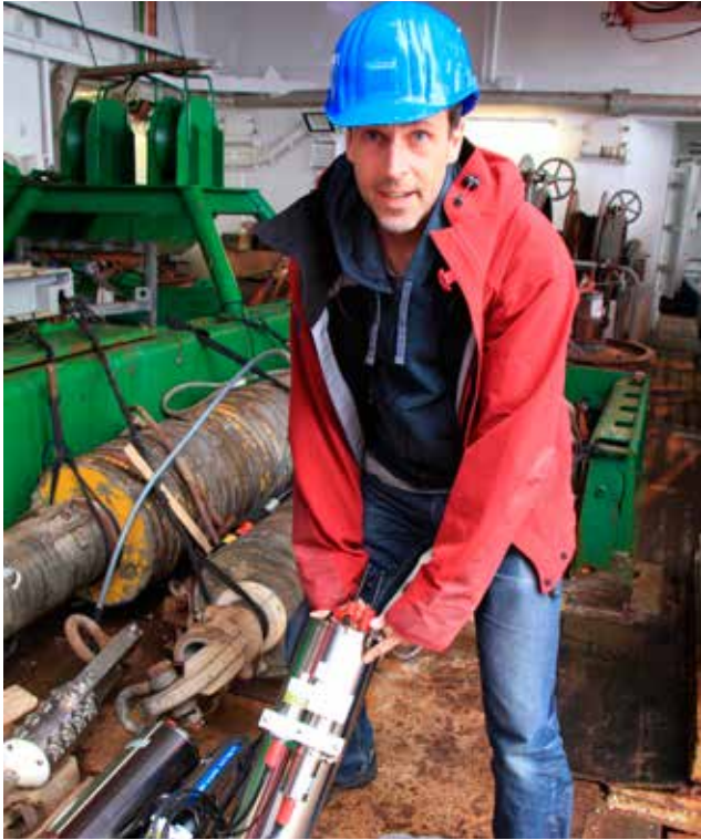
PhD candidate Pär Jansson holding a methane sensor that was installed to the ocean floor using the lander below. Photo: Kasia Zamelczyk.
