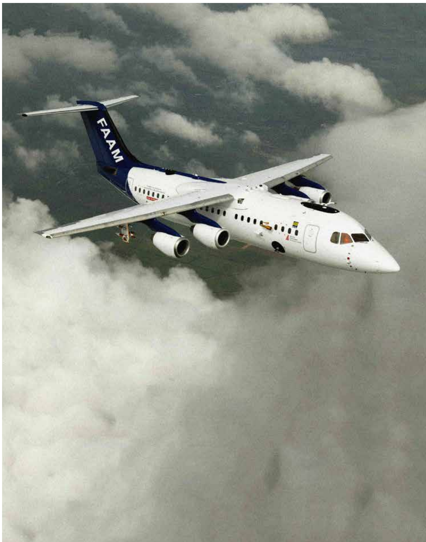
The modified BAe 146-301 large Atmospheric Research Aircraft (the ARA) is owned by the Natural Environment Research Council, UK. Photo: Facility for Airborne Atmospheric Measurements (FAAM)
