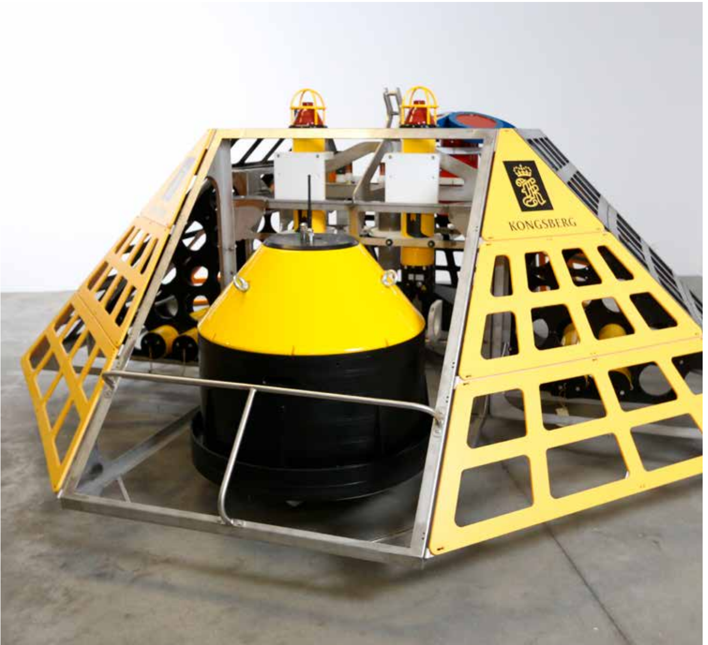
The observatories will include several instruments, be self-contained and wirelessly connected to the surface, sending data on a regular basis to CAGE scientists. Instruments will monitor methane release from the seabed to the water column as well as CO 2 ocean acidification and circulation. Photo: Kongsberg Maritime.
