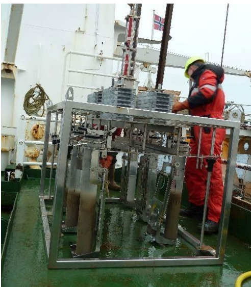
Figure 5: Multicorer after sediment collection.
