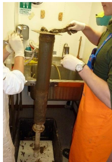
Figure 6: Slicing of the sub-bottom sediment layers.
