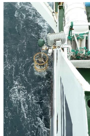
Figure 4: CTD SBE911plus (on the left) used for measuring physical properties of the water column.
