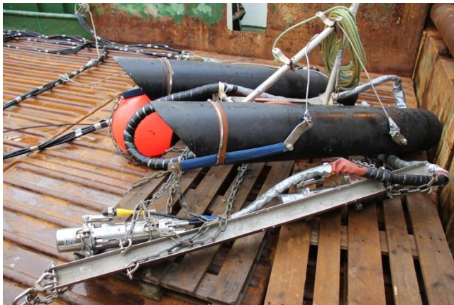
Figure 3.4.2 Mini GI gun used for seismic surveys during the cruise.
