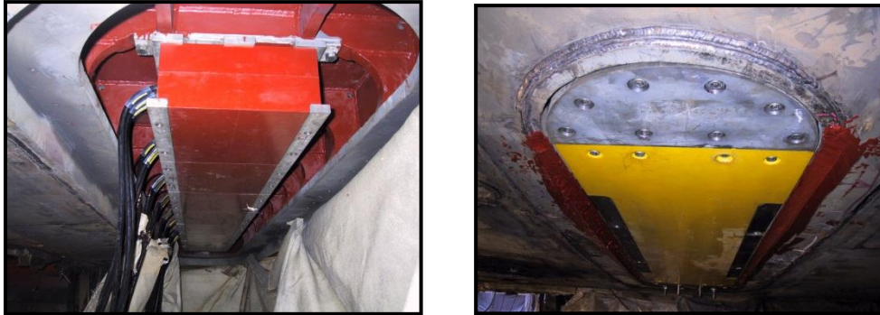
Fig. 3.2.1 – The multibeam system: Transmitters mounted in sea box (on the left) and the ice window (receiver) (on the right). Photo: Steinar Iversen, UiT.
