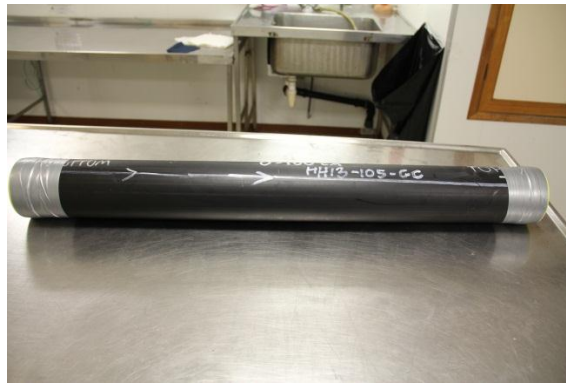
Figure.3.5.2 A 1 meter, labeled section from a gravity core
