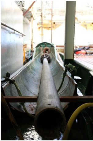
Figure.3.5.1 Gravity corer on Helmer Hanssen without core catcher and cutter.
