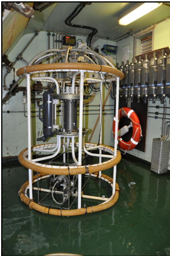
Figure. 3.3.1 CTD sensor set up onboard R/V Helmer Hanssen.
