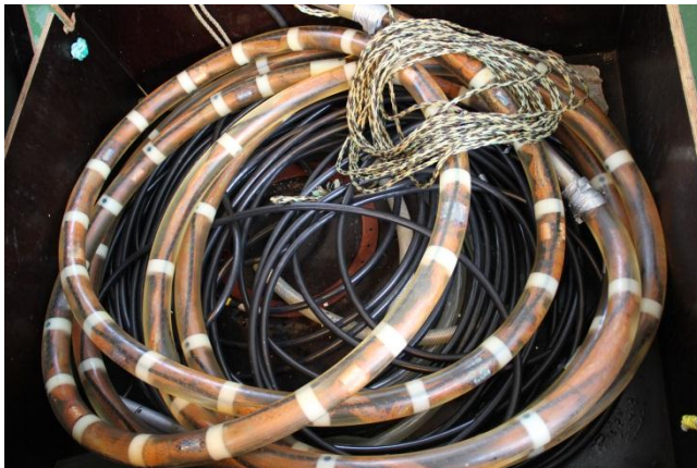
Figure.3.4.3 Single-channel streamer used for seismic surveys during the cruise.
