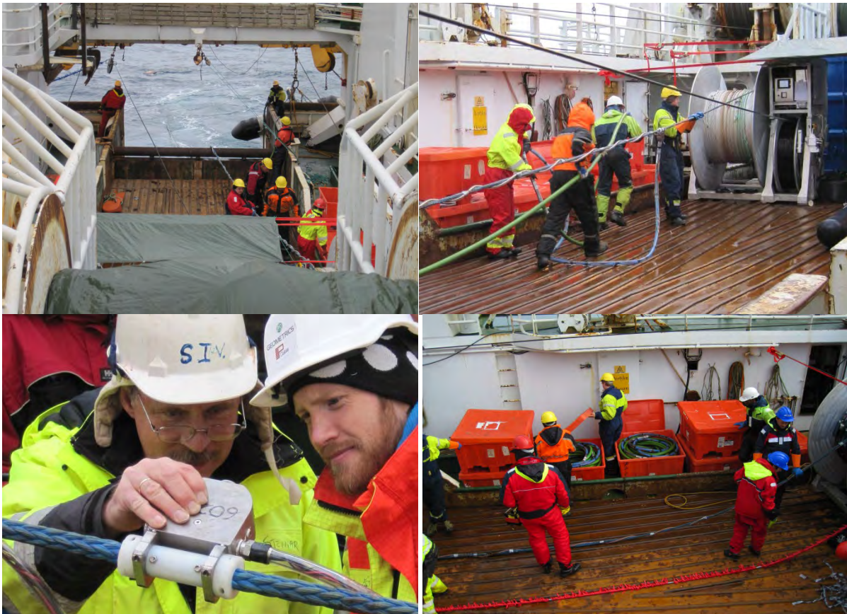
Figure 4: Images of the P-Cable system during deployment and recovery. Top left: the cross cable is being deployed, streamer sections are connected during deployment; top and bottom right: The cross cable is recovered and spooled back on the winch while streamers are disconnected from the cross cable. The small winch next to the cross cable holds the signal cable; bottom left: inspection of cross cable junction boxes during deployment and recover.
