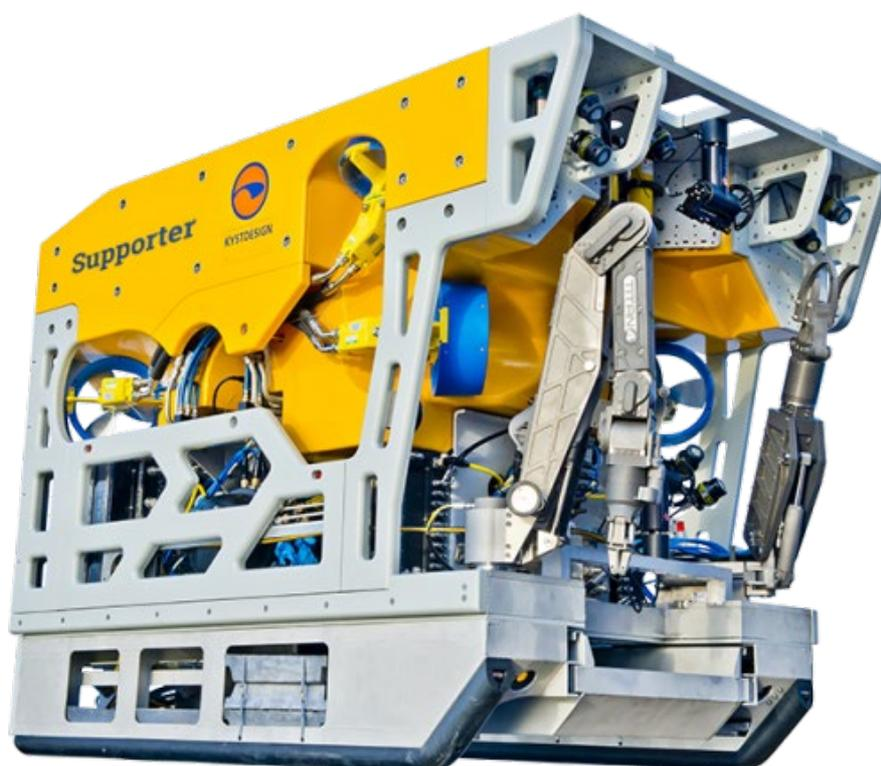
*Figure 3: The ROV Ægir6000 is a Kystdesign Supporter ROV rated to 6000 m water depth.*
