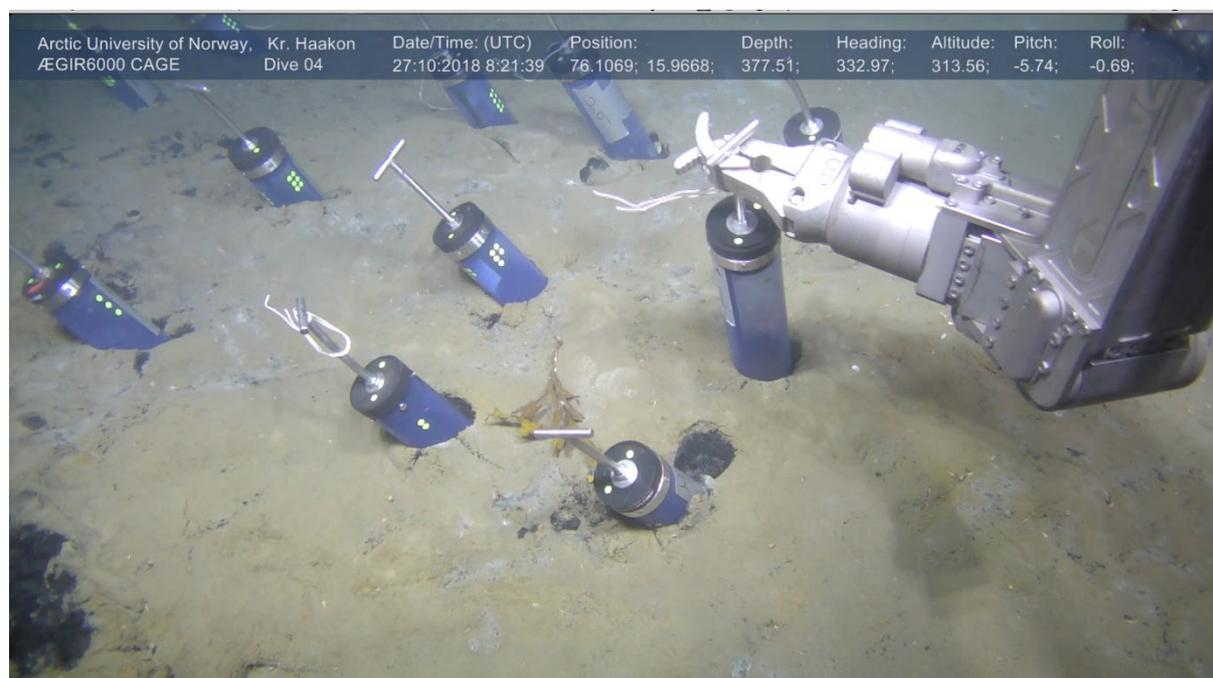
Figure 36: Sampling of densely spaced push cores with the ROV on gas hydrate pingo 3 site.
