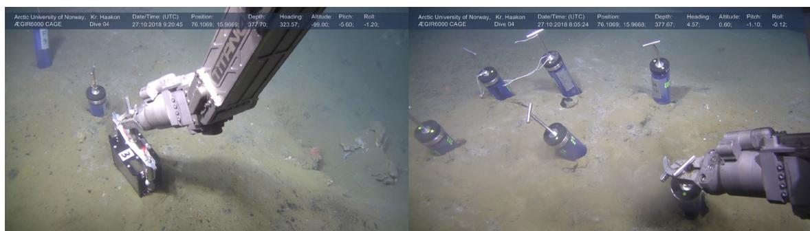
Figure 16: Dive 2 was dedicated to an intensive coring program with 20+ push cores for geochemical, sedimentological and microbiological investigations. Many push cores were closely spaced in areas with bacterial mats. A blade corer (left) can take a larger sample of the upper few cm of the seafloor and much better preserve the surface.
