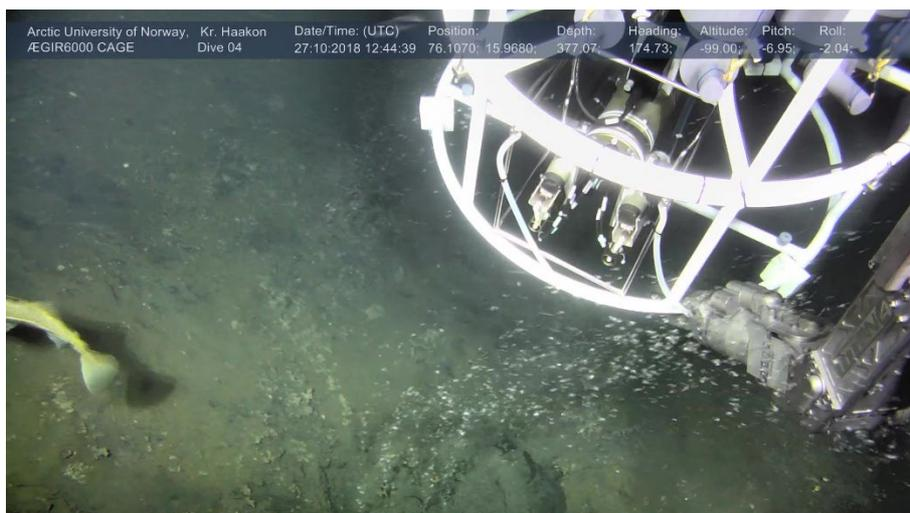
*Figure 9: CTD cast with ROV arm holding the rosette above the flare for water sampling at the source.*
