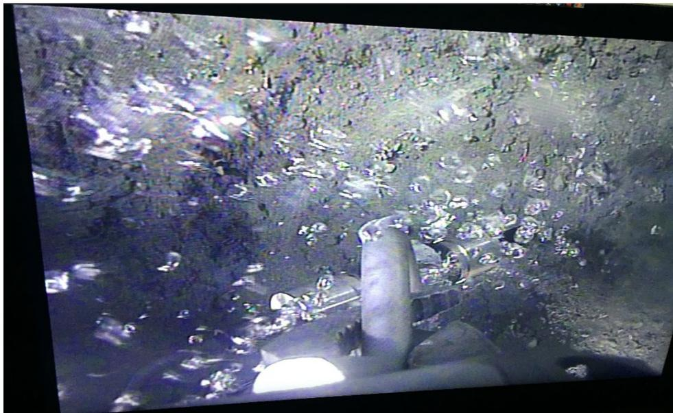
*Figure 38: Hydrophone placed by the ROV manipulator just above a seepage.*
