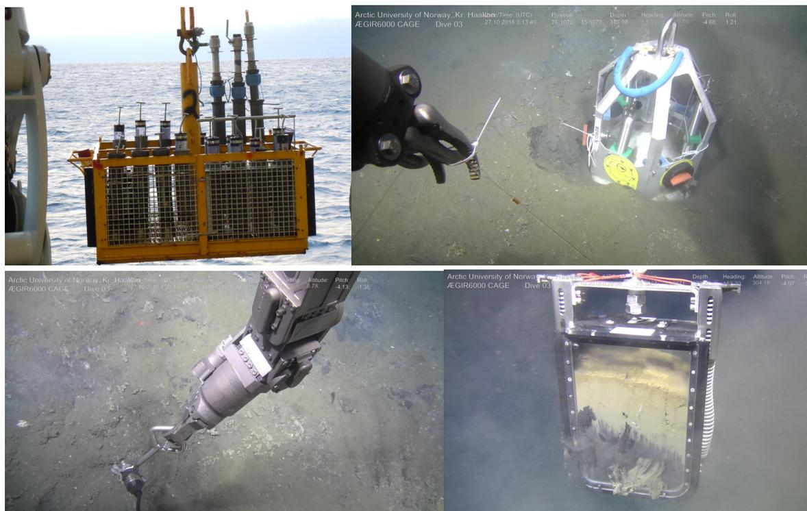
Figure 18: A basket was used to bring sampling tools down to and up from the seafloor (upper left). A gas sampler sampled gas twice over the most intensive gas seepage locations (upper right). We used a hydrophone to listen to the gas seepage (lower left). The blade corer is an excellent tool for obtaining an undisturbed seafloor sample (lower right).
