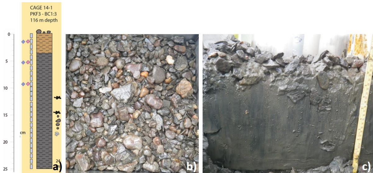
Fig. 5.15 From a water depth of 116m a box core with pebbles at the surface was taken. The uppermost layer of the core was composed of brown clay. The colour changed into grey clay at 4 cm. Black patches, pebbles and shell
