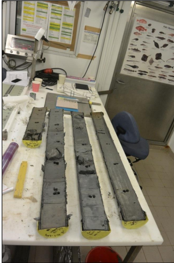
Figure 7.10 The core sections have been described and sampled. The coupled holes mark the sampled intervals.
