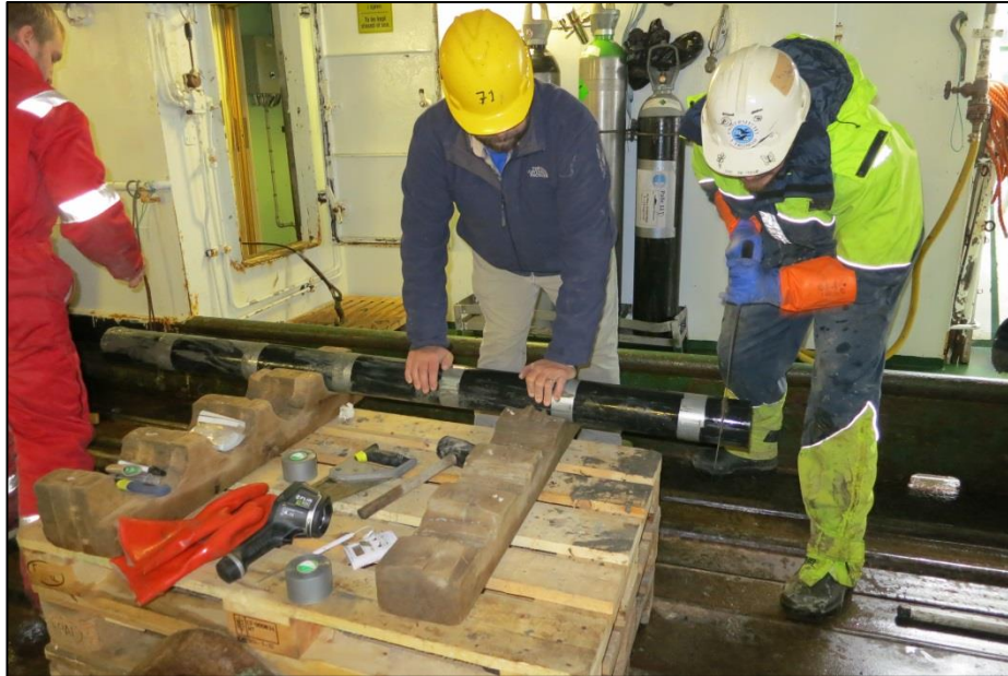
Fig. 7.7 The sections with no sediments are cut away from the plastic line lying on the pallets.
