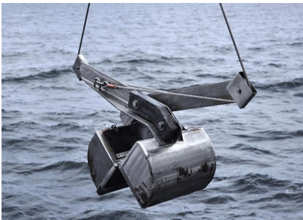
Fig. 6.4 Van Veen grab (0.1 m 2 ) in open mode (Photo, private)
