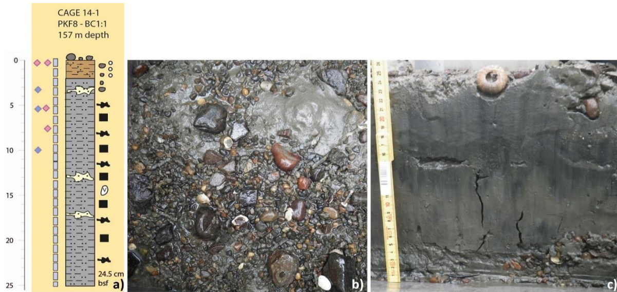
Fig. 5.17 From the site PKF 8 a box core with brown mud, sand and gravel at the surface was recovered from 157 m water depth. The surface facies was soupy below the pebble layer. The pebbles were subrounded in shape, had a diameter of < 2cm, and were composed of different lithologies. The sediment changed into grey clay 2 cm below the surface. Black patches, sand lenses and compact, stiff areas occurred sommonly within the grey clay. A void with a diameter of 1.5 cm was found in 14-15 cm depth below the seafloor surface. a) shows the sediment log of the box core.
