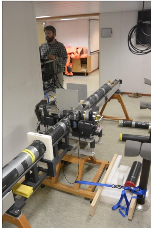
Figure 7.8 The core sections are logged in the Multi-Sensory Core Logger (MSCL).
