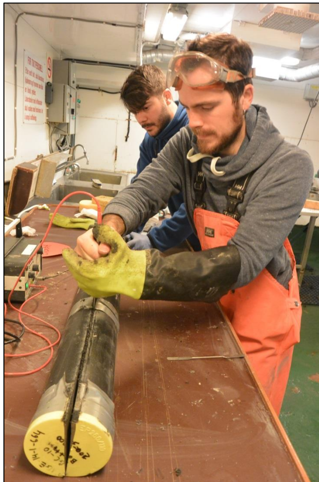
Figure 7.9 The sawed core section is split using the osmotic knife.
