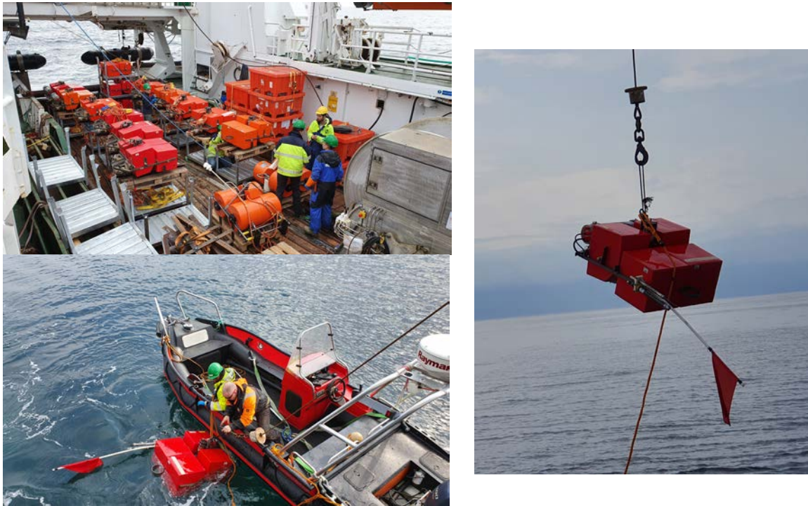
Figure 5: top left: OBS spread out over the Helmer Hanssen deck; bottom left: weather conditions allowed to use the working boat to snatch OBS from the water and tow them to the ship; right: OBS on the hook of the crane being recovered.
