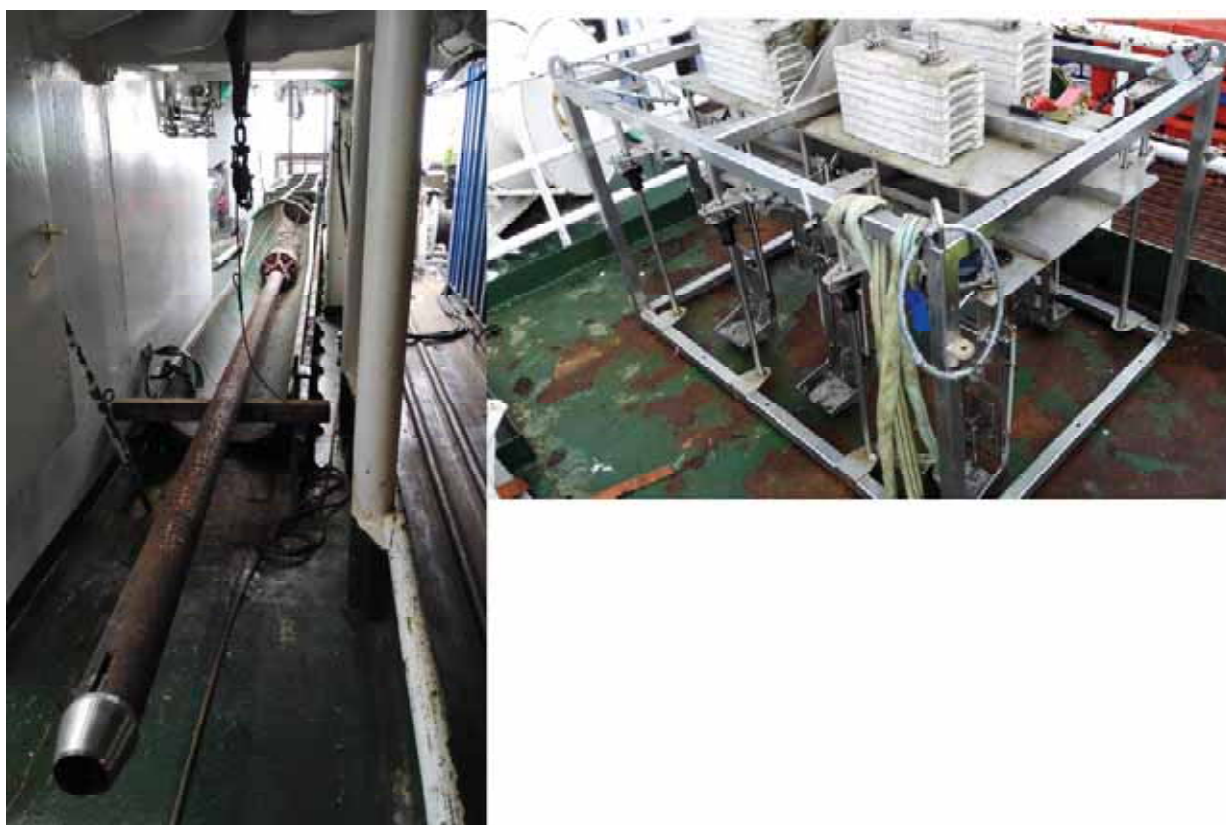
Figure 13. Gravity corer (left) and multi-corer (right) used to collect sediments at KKLP.
