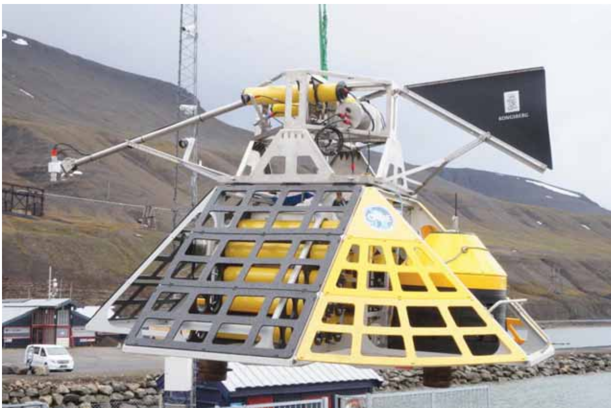
Figure 34. The K-Lander with Launcher system is lifted on board Helmer Hanssen using the HH Crane and onto the Geology deck.
