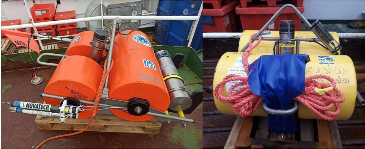
*Figure 3: Ocean-bottom seismometers of UiT (left) and AWI (right).*
