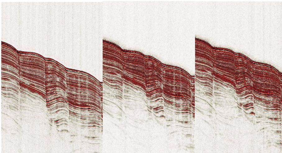
Figure 8: From left to right: example of stack, Kirchhoff migrated, and amplitude equalization results for line 3.
