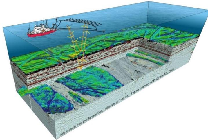
*Figure 2: Schematic sketch an acquisition principle of the P-Cable high-resolution 3D seismic system.*
