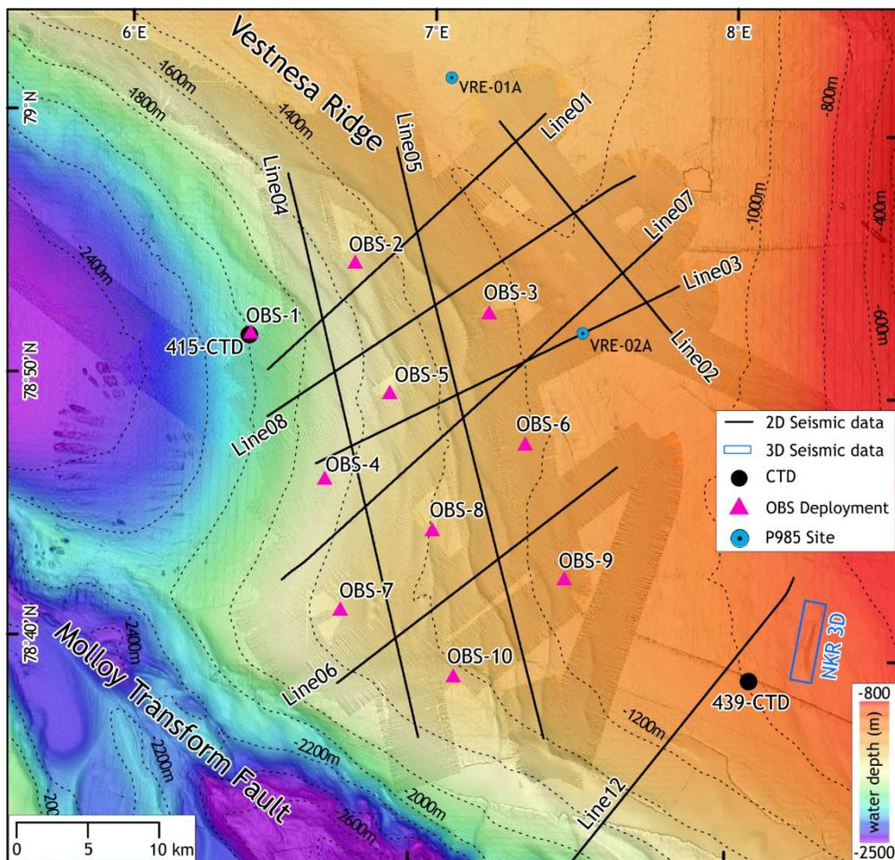
Figure 5: Overview figure showing OBS deployed and seismic data acquired during this expeditions.
