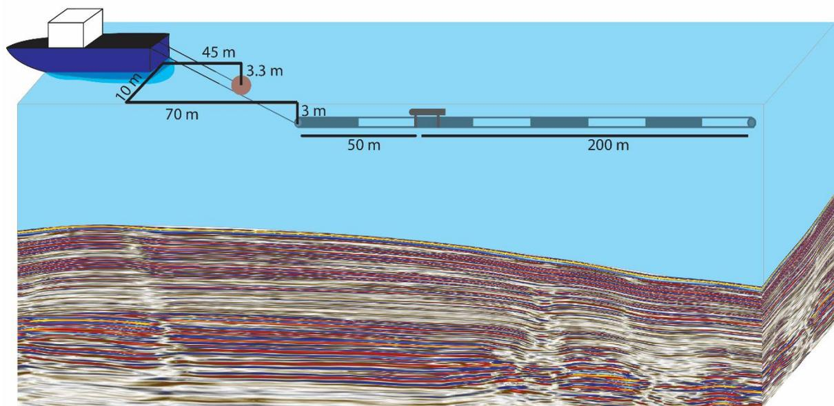
Figure 6: Acquisition geometry of the 2D multi-channel seismic streamer. Notice that in this cruise we used 12 streamer sections. Hence, the active section was 300 m instead of 250 m. The distance of the source behind the vessel varies but can be obtained from nav track records of the gun and aft Seatrack antennas.
