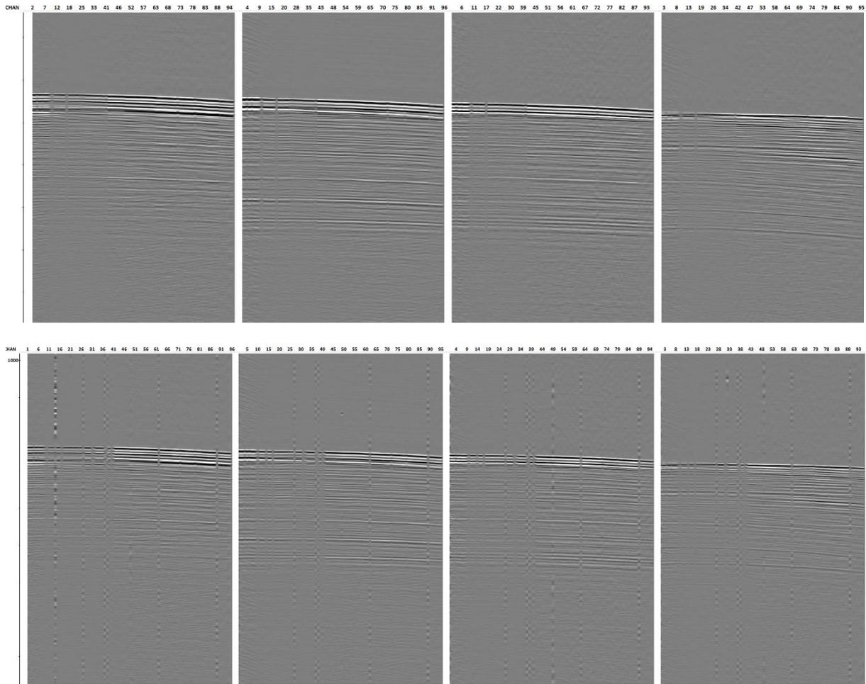
Figure 7: Shot gathers after (above) and before (below) burst noise removal for line 12.
