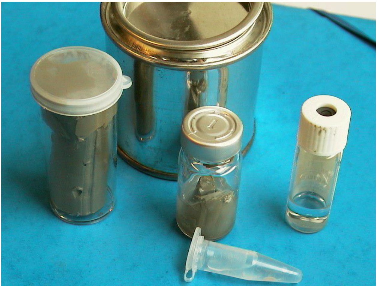
Photo (Troels Laier, GEUS, Copenhagen). Vials for pore water (exetainer and Eppendorf tube), crimp vial for methane samples, and jar for TOC samples.
