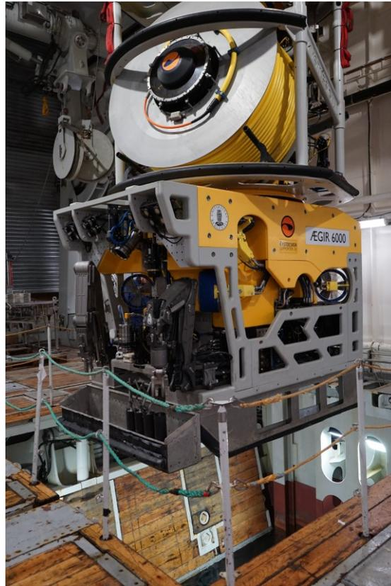
*Fig. 16. ROV ÆGIR6000 and TMS system, ready to be deployed from the moon pool.*
