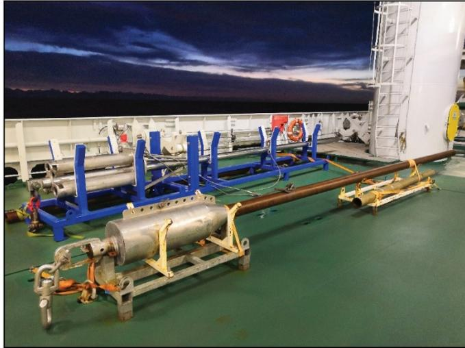
*Fig. 11. Gravity corer used during the cruise. The barrel is 6 m-long and hosts a plastic liner with outer diameter of 12 cm.*
