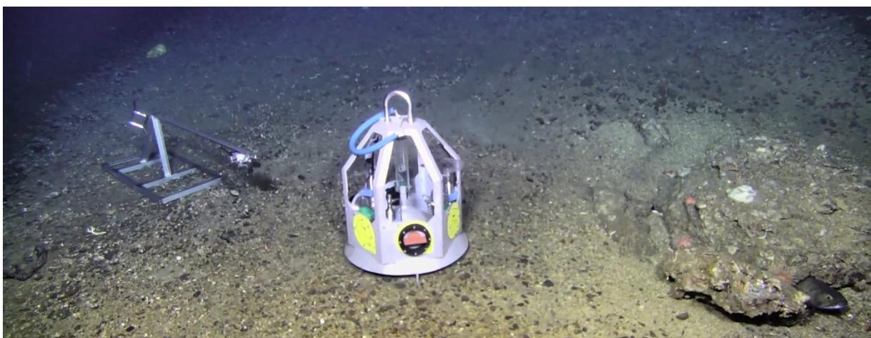
*Fig. 24. Bubble catcher (middle) and hydrophone (left)*
