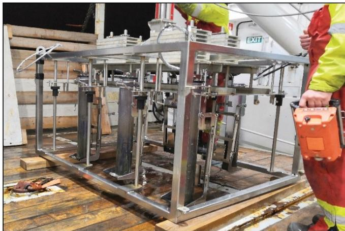
*Fig. 12. Multi corer (frame 180x125x100cm) hosting 6 core liners (inner diameter 10cm, length 80cm).*
