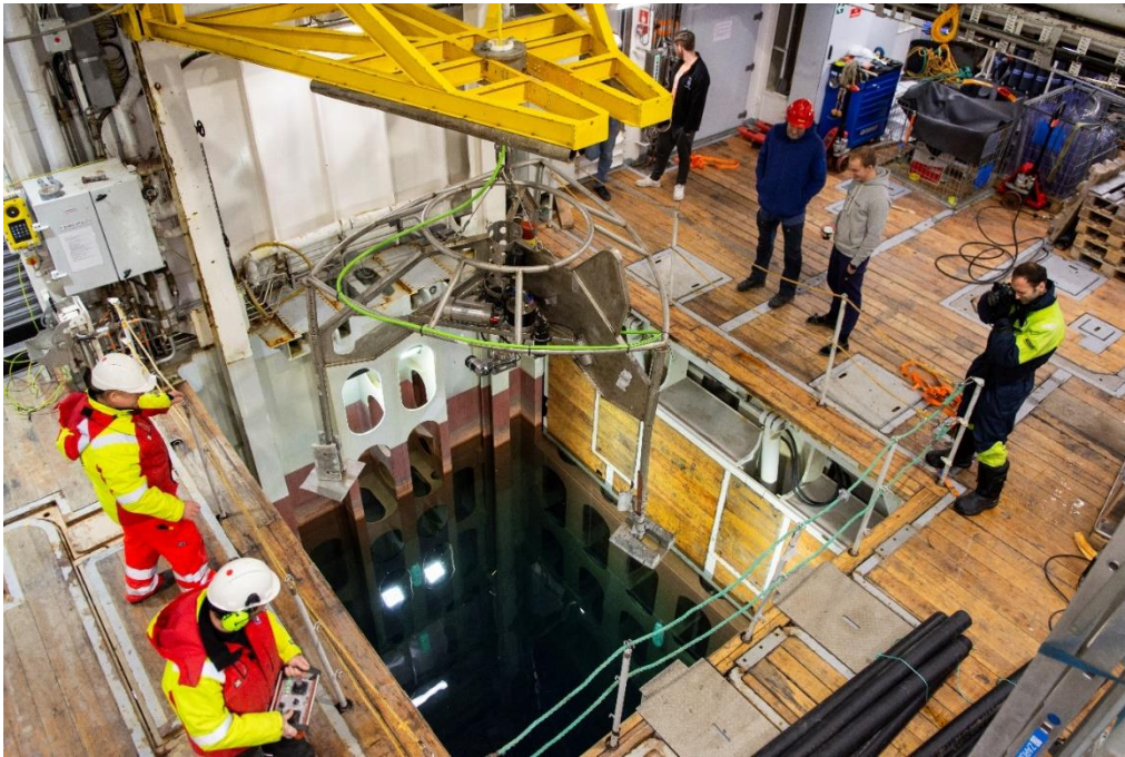
Figure 15. CAGE 20-8-KH04 – CamPod video system is lowered through the Moonpool.
