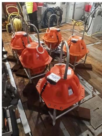
Figure 10 Ifremer Ocean Bottom Seismometers
