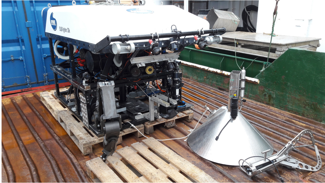
Figure 3: The remotely operated vehicle 30k on Helmer Hanssen's deck with the gas sampler and the claw for geological research.
