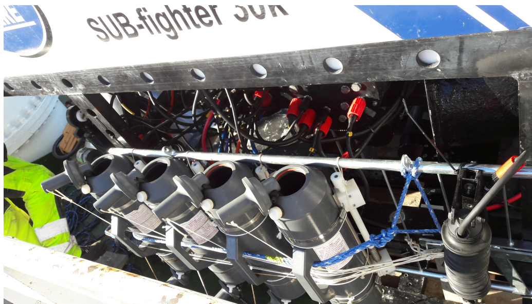
Figure 8: A four-Niskin bottles module installed on the port side of the ROV and triggered with a linear actuator.
