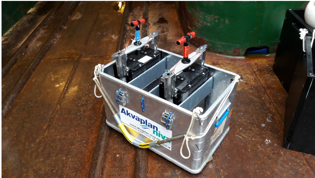
Figure 10: The blade core transport case with capacity for four samplers at a time.
