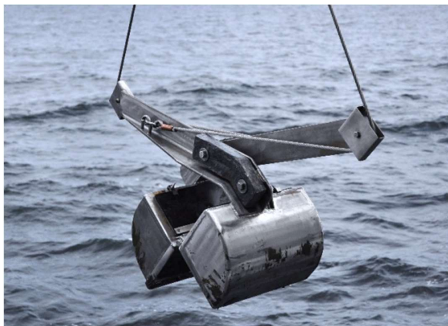
Figure 8: Van Veen grab in open mode from RV Helmer Hanssen (Photo E. Åström).
