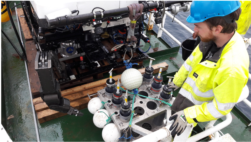
Figure 11: The pushcore rack was hung from the hook at the ROVs boom and then the arm held it from the Tbar installed for this purpose.
