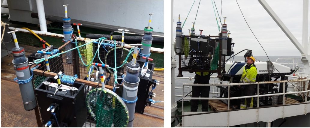
Figure 7: The cage was well equipped with blade cores, push cores and nets, four of each, a time lapse camera and markers.
