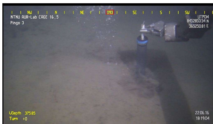
Figure 9: Push core sample take by ROV directly at a flare in the Storfjordrenna Pingos.
