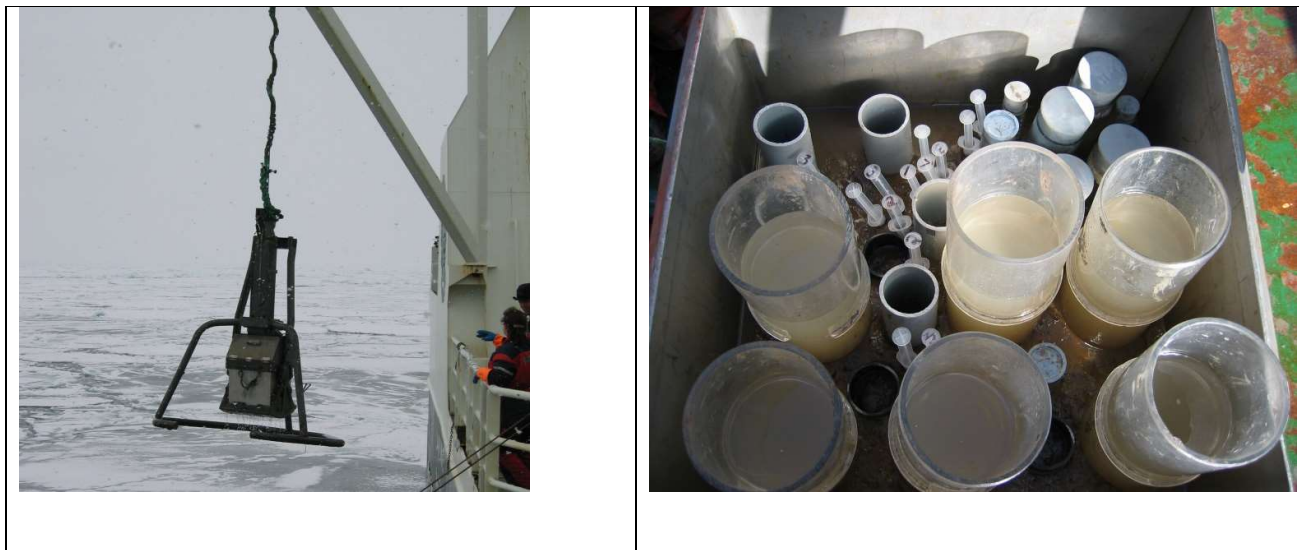
Figure 10: A box core in action from RV Helmer Hanssen, and subsampling of a box core sample (Photos: M. Carroll).
