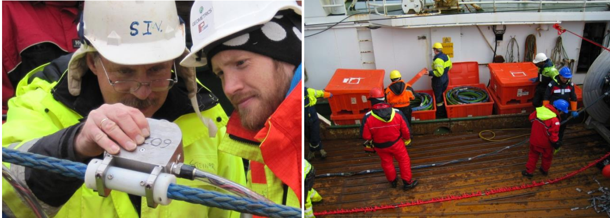
Figure 4: Images of the P-Cable system during deployment and recovery. Top left: the cross cable is being deployed, streamer sections are connected during deployment; top and bottom right: The cross cable is recovered and spooled back on the winch while streamers are disconnected from the cross cable. The small winch next to the cross cable holds the signal cable; bottom left: inspection of cross cable junction boxes during deployment and recover.
