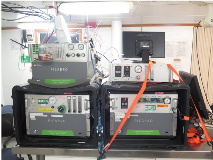
Figure 5. PICARRO CDRS system for surface waters and lower atmosphere
