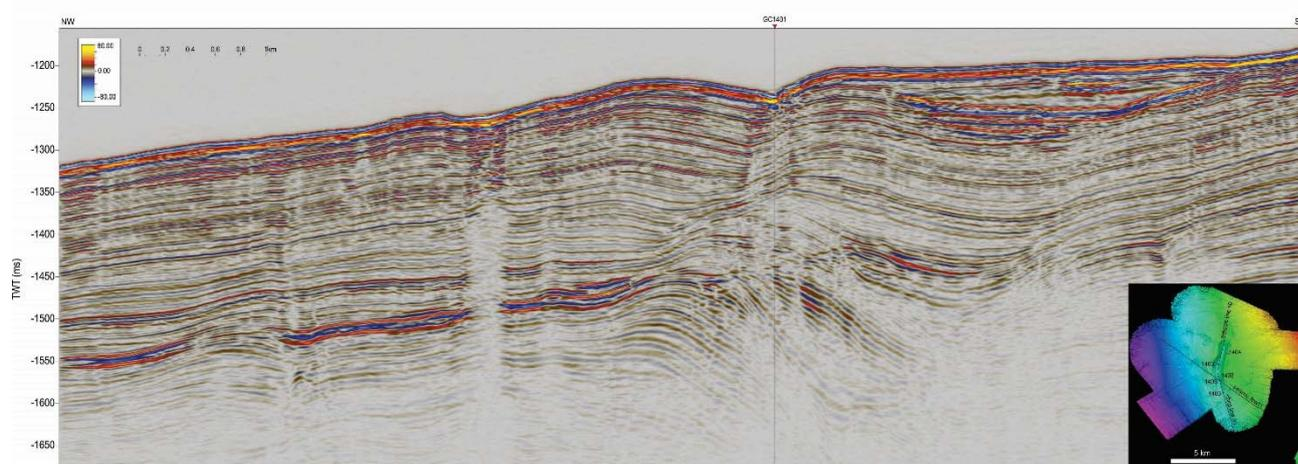
**Figure 19. Seismic profile Cage 17-5\_011 across sediment core Cage 17-5\_1401GC that contained massive gas hydrate.**
