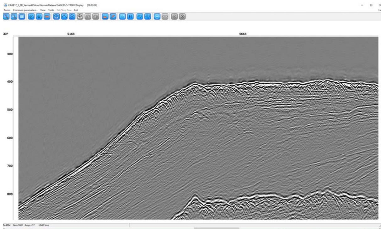
Figure 11. Western Svalbard Margin Cage 17-5\_WSM2D\_013: stacked and debubbled using demultiple.
