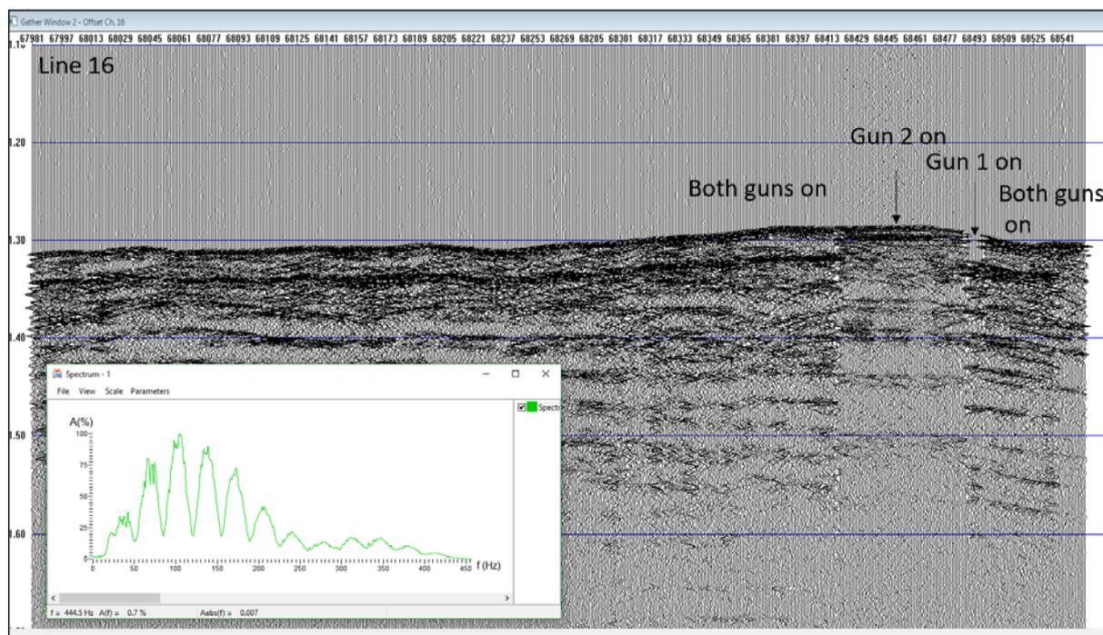
**Figure 12. Western Svalbard Margin seismic line Cage 17-5\_WSM2D\_016 showing problem with unsynchronized airguns.**
