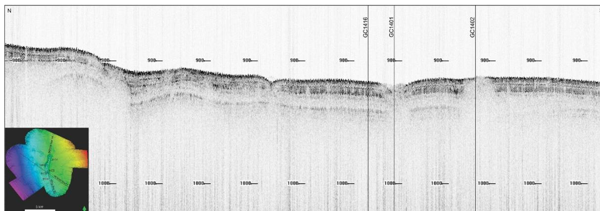
**Figure 20. Chirp profile 030 (same location as seismic line 010) showing GC location Cage 17-5\_1401GC, which contained massive gas hydrate.**
