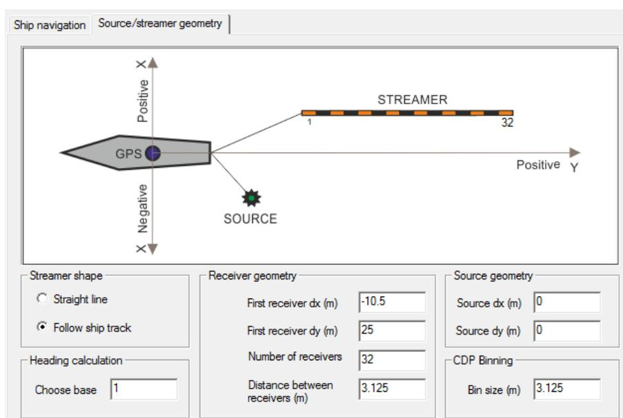
**Figure 5. Geometry of the 2D seismic survey during CAGE17-5 cruise. The gun position is used as a reference point for streamer geometry calculation.**
