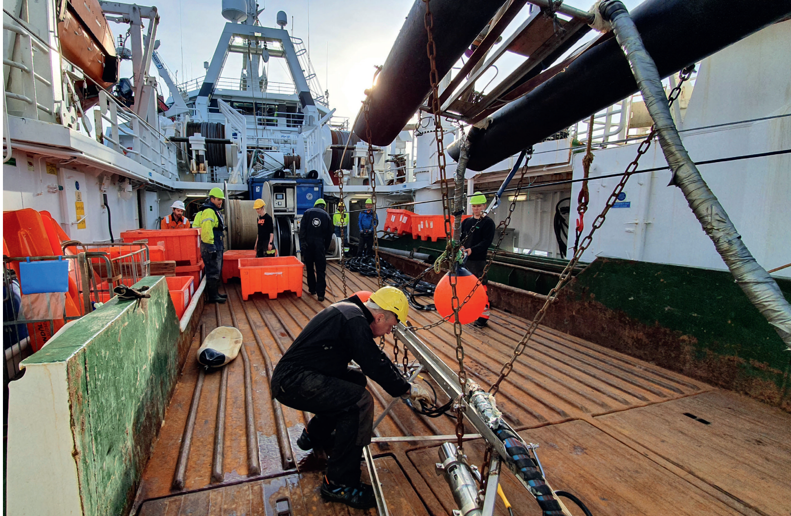
Technician Steinar Iversen makes a final check of the airgun system before deployment. Photo: Stefan Buenz.
