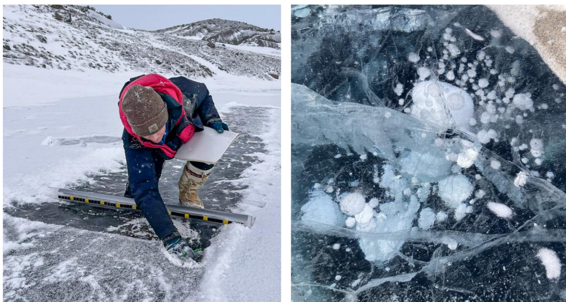
Figure 18. Left: LB performing methane ice-bubble survey on lake G13. Right: Cluster of methane bubbles trapped in lake ice. Photo credit: left, Marie Bulínová; right; Arthur Fouillé
