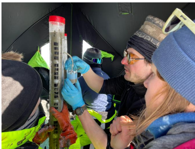
Figure 12. Example of sampling of bottom lake water from above the sediment/water interface inside a core liner and destined for dissolved gas analyses. Photo credit: Joost van Genuchten
