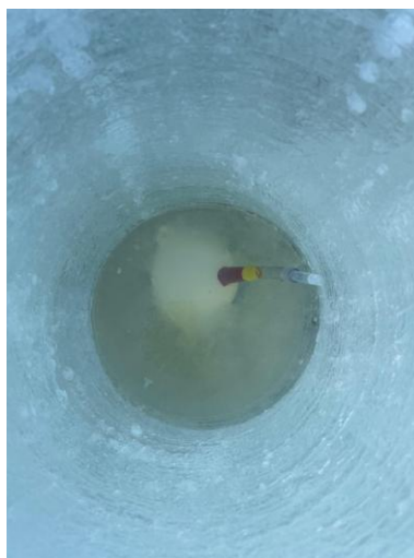
Figure 15. Photo of an inverted funnel inside a lake borehole. Visible is only the funnel and tubing without the syringe and valve attachments.
