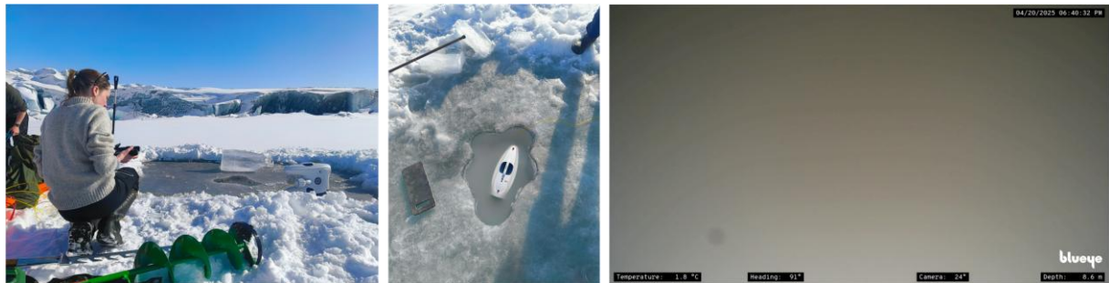
Figure 17. Deployment attempt of the BlueEye ROV on lake TB1. Left: Team next to deployment borehole – Russell Glacier visible in the background. Middle: Deployment borehole with the top of the BlueEye ROV visible. Right: Screenshot of (absence of) visibility in lake water column (TB1 lake, 2025.04.20).
