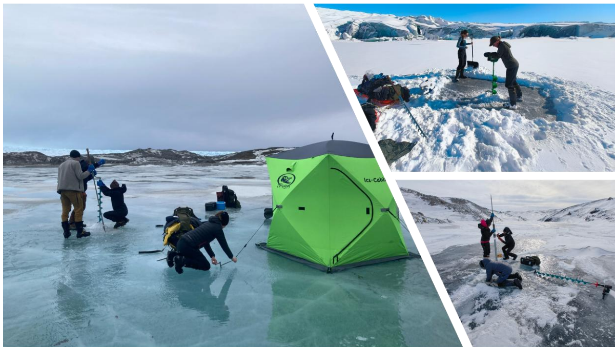
Figure 8. Left: Ice borehole created using hand auger and ice pick on lake G23 and installation of science tent; surface of Russell Glacier visible in the background (2025.04.09). Top-right: Borehole created using an electrically powered auger (IonIce Fishing instrument – courtesy of Dr. Jasmine Saros) on lake TB1 (2025.04.13) – ice margin of Russell Glacier visible in the background. Bottom-right: Sediment corer with liner deployment into a borehole on lake G13 (2025.04.04) – also visible is ice-auger connected to electrical drill used to create the borehole and glacier moraines in the background.
