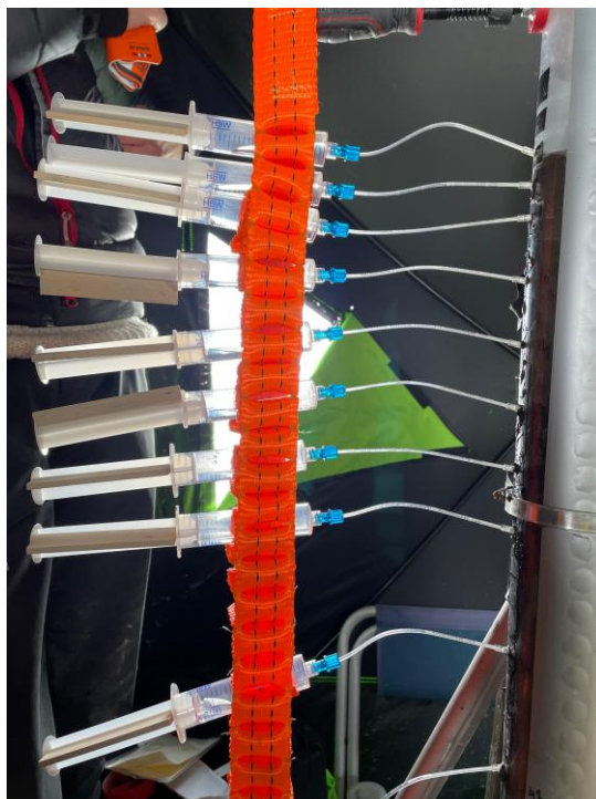
Figure 11. Example of porewater extraction inside the field tent. Photo credit: Joost van Genuchten
