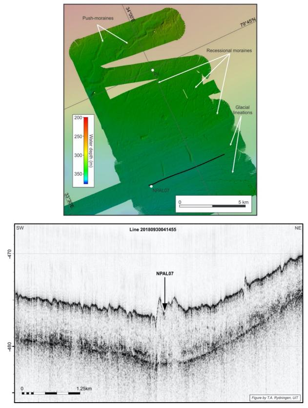
Figure 3: Figure 4: Multibeam bathymetry and selected seismic profile at the NPAL07 site.
