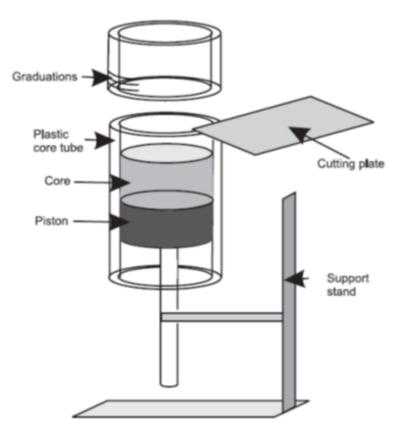
Figure 14: Schematic representation of a stand with a piston for sediment slicing (Murray 2006).
