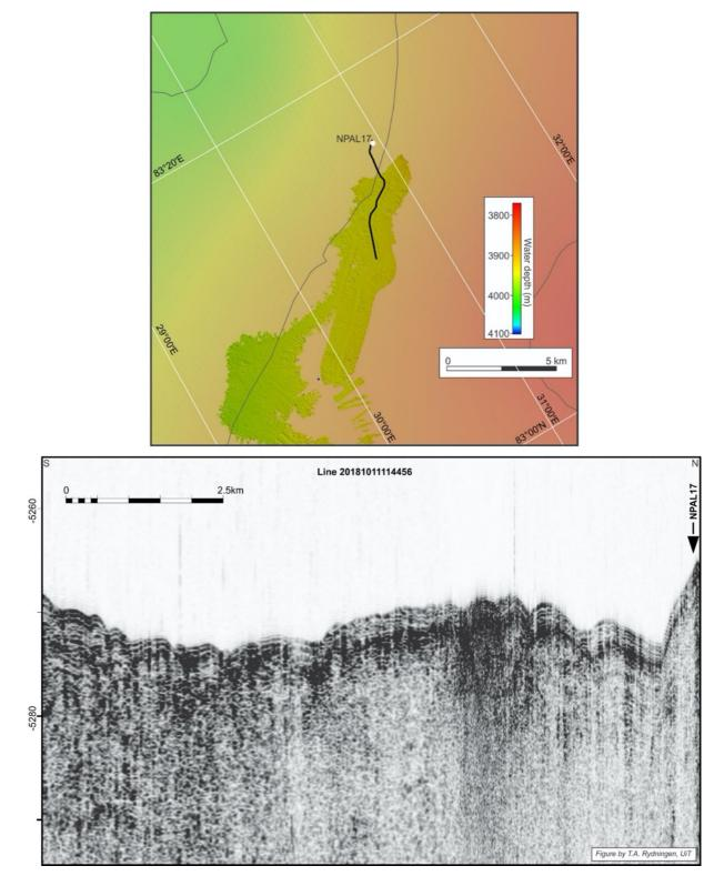
Figure 9: Multibeam bathymetry and selected seismic profile at the NPAL17 site.
