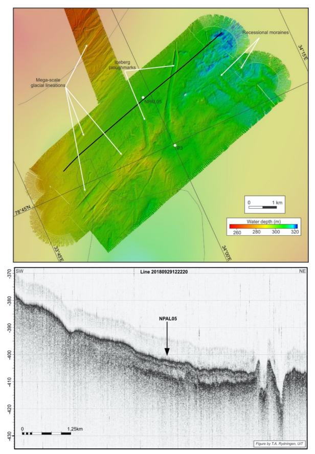
Figure 2: Multibeam bathymetry and selected seismic profile at the NPAL05 site.
