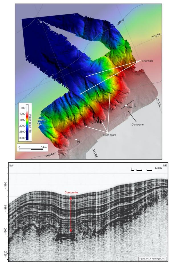
Figure 8: Multibeam bathymetry and selected seismic profile at the NPAL14 site.
