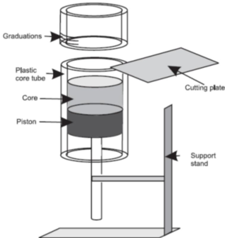
Figure 14: Schematic representation of a stand with a piston for sediment slicing (Murray 2006).
