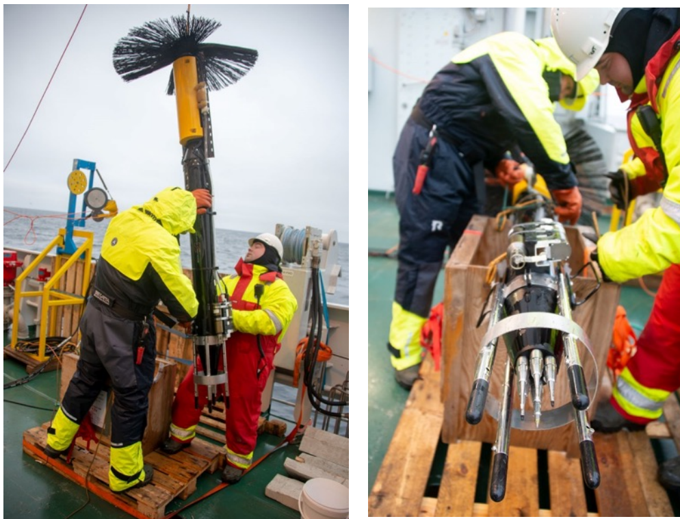
Figure 10. (Left) The VMP profiler during deployment. The brushes provide the drag for the profiler. Drag, together with the buoyancy elements (yellow) set the nominal sink velocity of the profiler. Note the recovery line attached to the cable which allows recovery by a crane without damaging the cable. (Right) The hydraulic line-puller.
