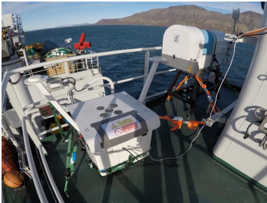
Figure 20. Windcube LIDAR and HATPRO microwave radiometer installations. The equipment was installed towards the aft of Deck 6, Port side. Port side gallow can be seen in the background.
