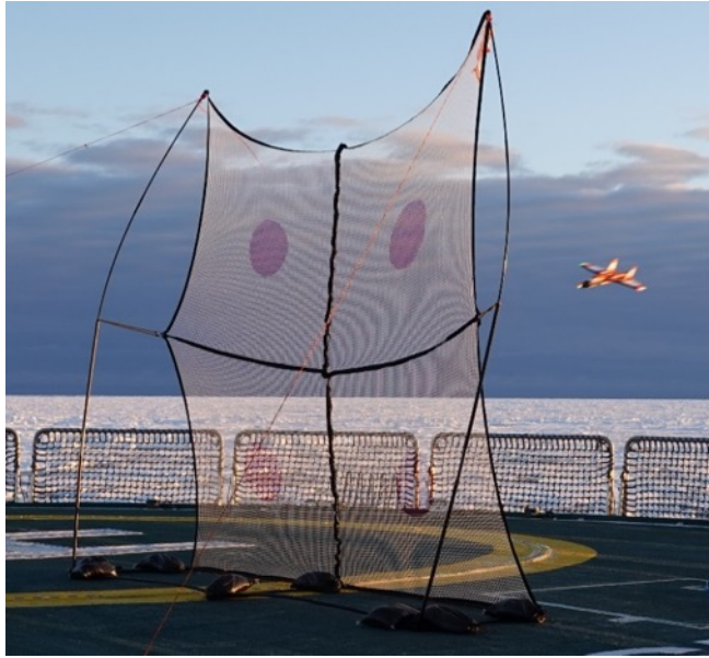
Figure 19. SUMO RPAS coming in for a net landing. The net is secured with sandbags and rope.
