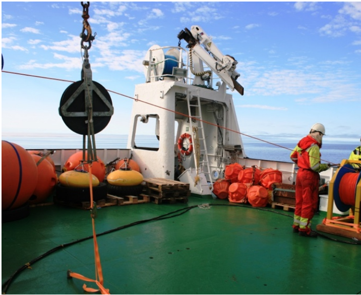
Figure 8. The set-up, on deck, of the VMP microstructure profiling system. The hydraulic winch (above); the cable is fed through a block supported by the crane in the middle. The block is fastened by straps to the deck to avoid swings due to wind and ship's roll. The tether then is fed into the line-puller (right) fastened to the ships' railing. In addition to the winch operator, a second person observes the cable in water during the deployment, and assists with deployment and recovery.
