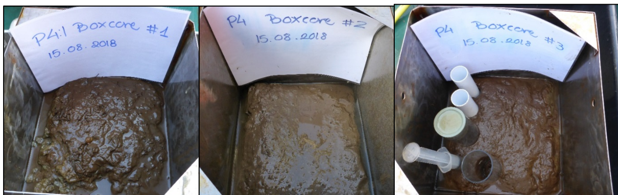
Figure 21: Sediment surface from station P4 approx. 330 m deep. Reddish/brown on top, very fluffy/soupy sediments. Iron deposits visible around grains in deeper layers. Darker brown sediments down core.
