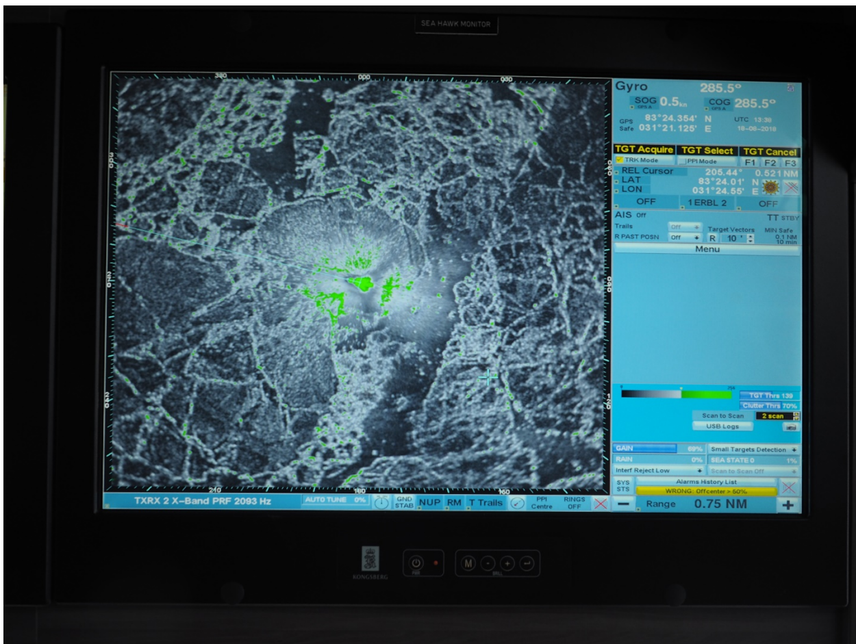
Figure 9. Ice station 2 (PICE1) ice floe on ice radar. The range 0.75 NM stands for the distance from the center to the left/right edges of the screen.
