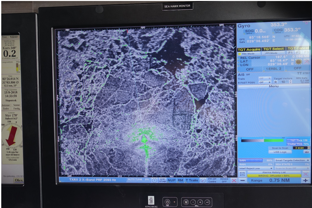
Figure 11. Ice radar image of station 3 and 4 (SICE2b) ice floe. The range 0.75 NM stands for the distance from the center to the left/right edges of the screen.
