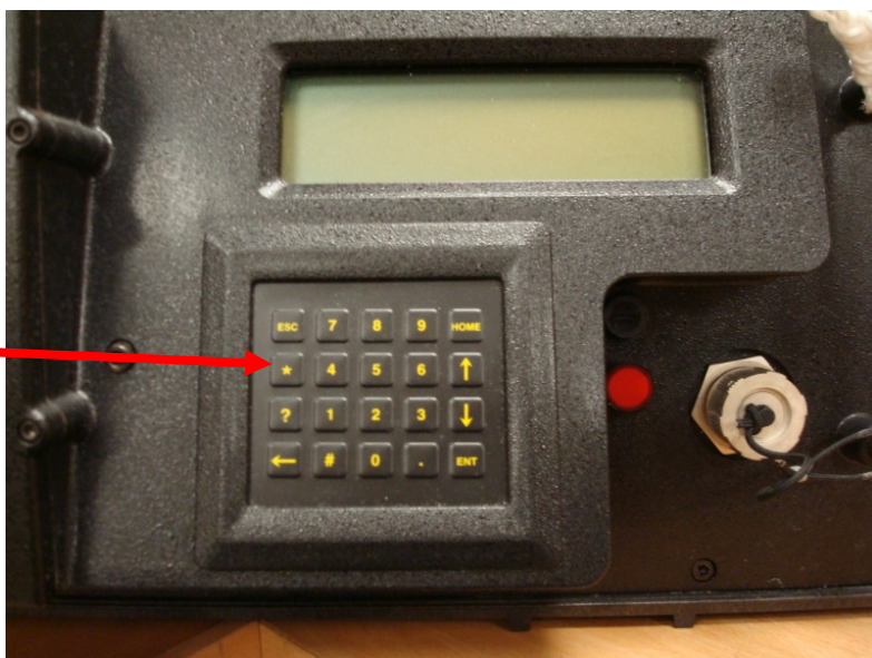
Fig. 1 Display and buttons of the Turner Design AU10 Fluorometer, * button is indicated by the red arrow
